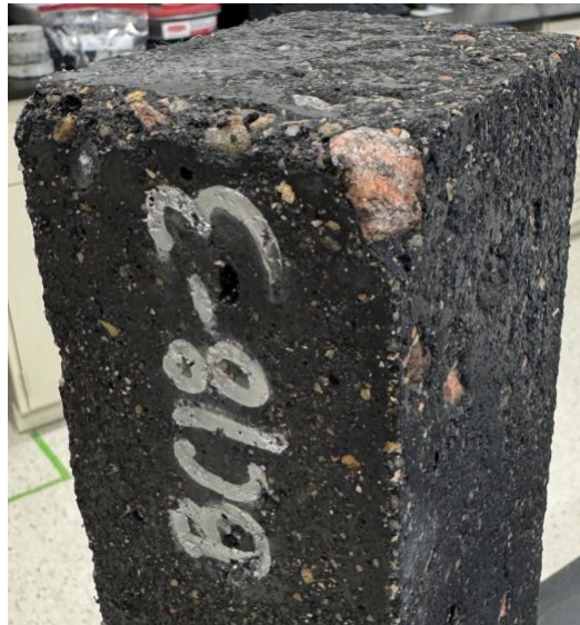
Figure 5.8 PW BC Concrete Mass Loss at 170 FT cycles
