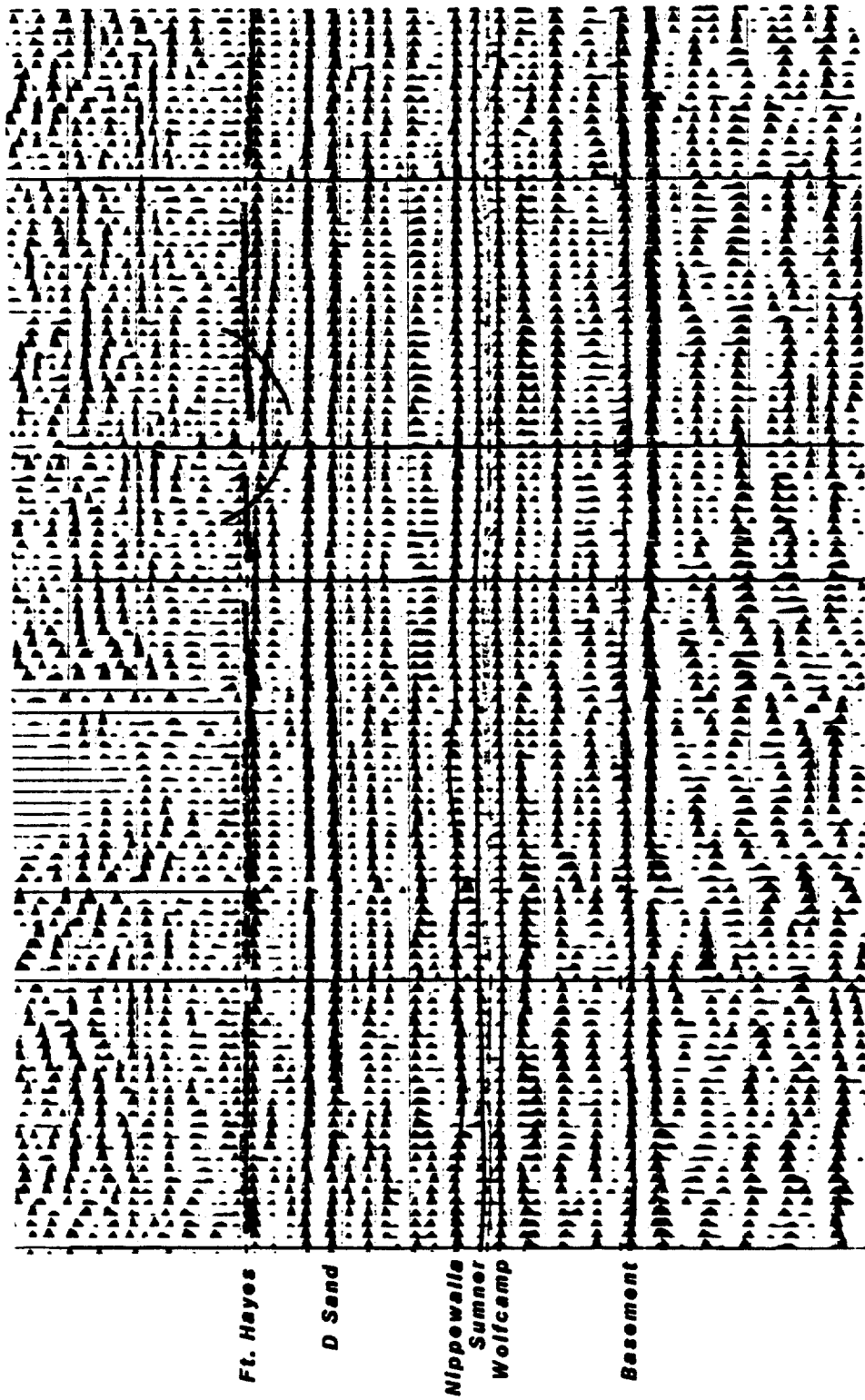
Fig. 23 Portion of line 4 showing Nippewalla First Salt dissolution and Niobrara listric faulting.
