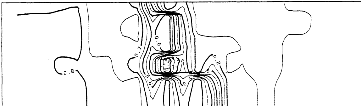
Figure 6.7. Saturation Contours of Run Number 4. Water Flood. Low Permeability sand.
