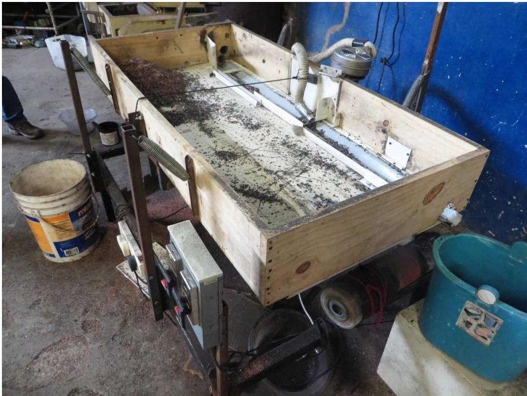
Figure 3.3 Example of a densiometric table built by an e-waste worker in Buenos Aires. (G. L. Clinckspoor & Zulaica, 2022)
