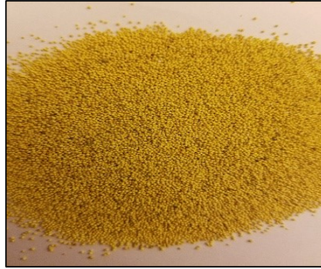
Figure 3.21: Picture of the 20/40 ULW ceramic used in the experimental study.
