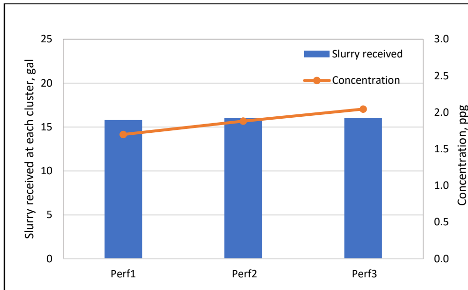
Figure 4.52: Proppant and slurry distribution between the perforation clusters at a slurry velocity of 13.7 ft/s and an injected proppant concentration of 1.79 ppg.
