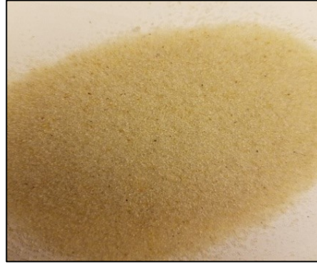
Figure 3.18: Picture of 40/70 white sand used in the experimental study.
