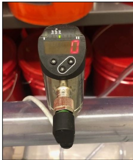
Figure 3.10: Picture of one of the pressure transducers used in the experimental apparatus.
