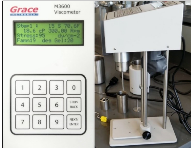
Figure 5.1: Picture of a M3600 Fann Viscometer used to measure the rheological properties of fracturing fluid.
