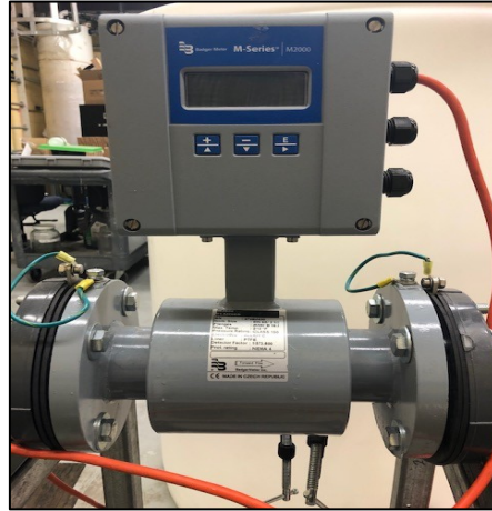
Figure 3.5: Flow meter used to measure the slurry flow.
