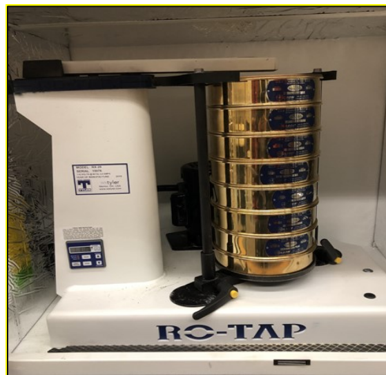
Figure 3.15: Picture of the sieve shaker used to perform the sieve analysis.
