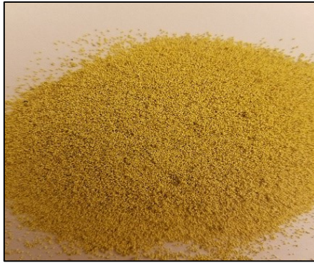
Figure 3.24: Picture of the 40/70 ULW ceramic used in the experimental study.
