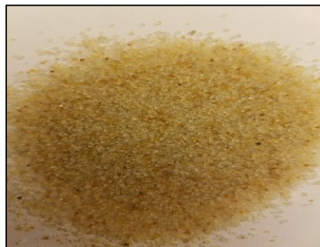
Figure 3.14: Picture of 20/40 white sand used in the experimental tests.
