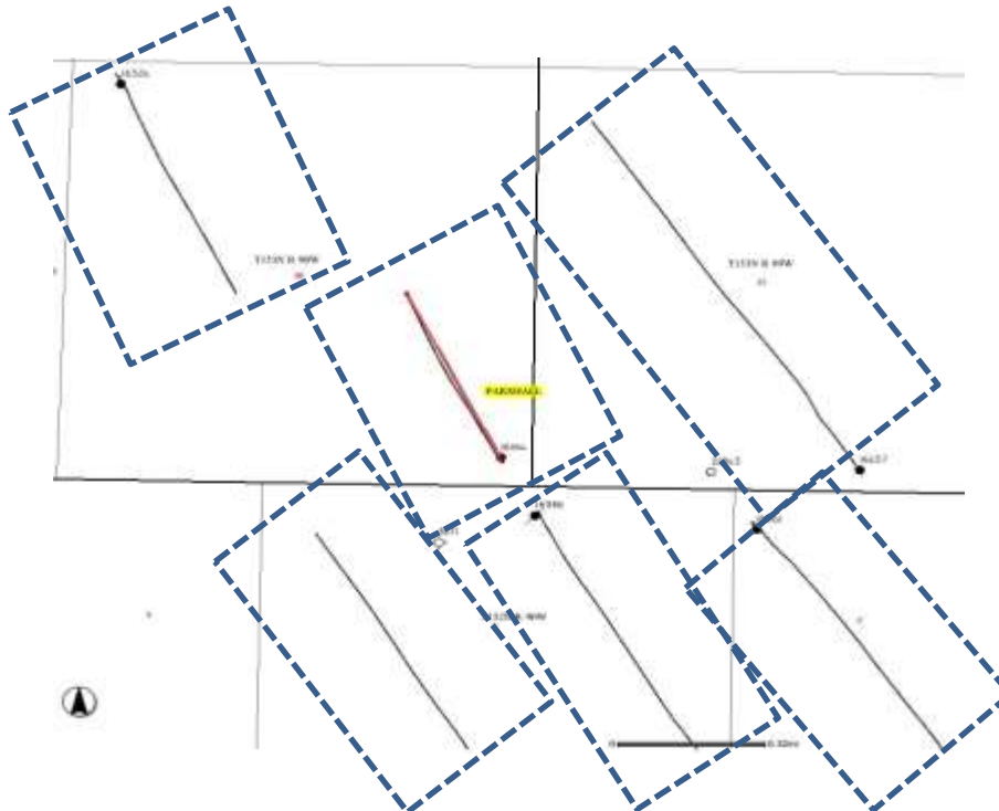
Figure C.1: Well drainage area determination: Broken line rectangles around solid black lines represents the Stimulated reservoir volume.
