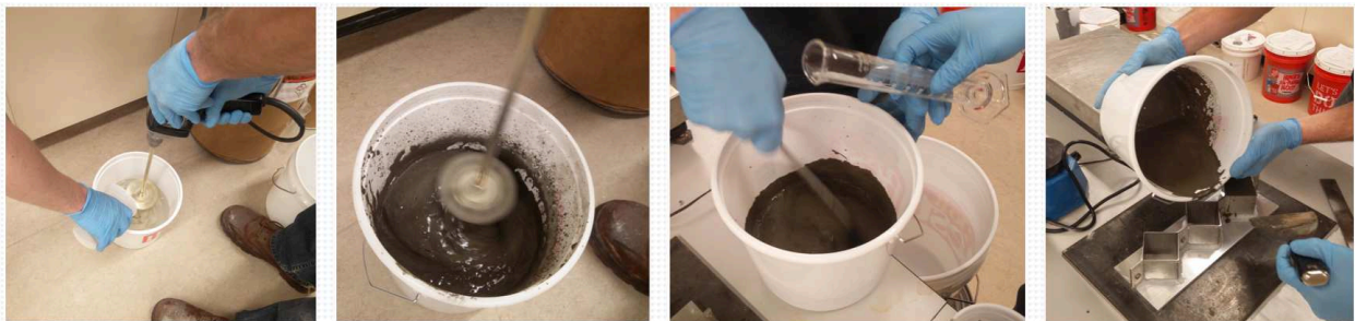
Figure 4.1 Photos of grout mixing process and pouring into cubic molds
