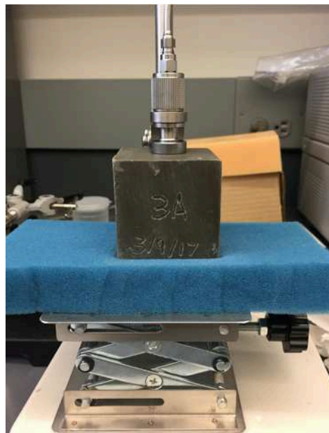
Figure B.3 Cubic grout specimen placed in contact with the OC probe by use of a laboratory lift and foam block to maintain firm pressure
