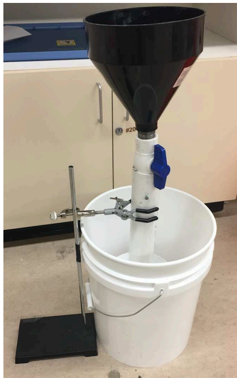
Figure 4.4 Photo of funnel used for pouring mixed grout into electrical conductivity test tubes
