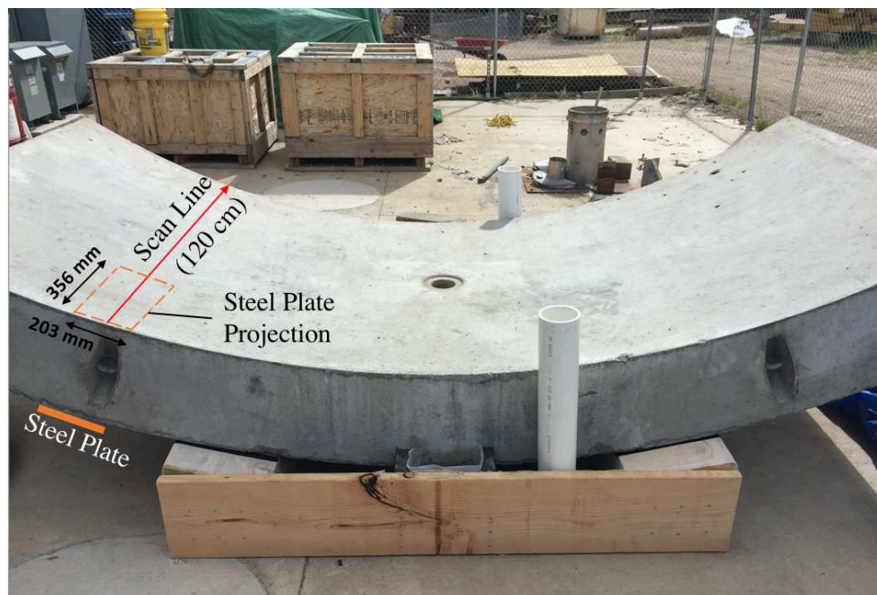
Figure 5.5 Picture of the segment on top of support frame used for penetration depth testing
