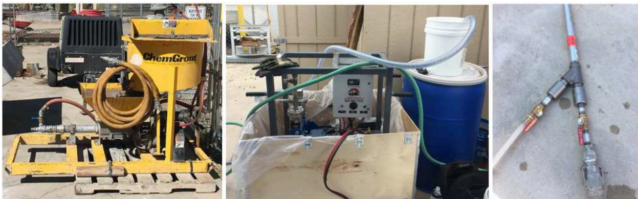
Figure 5.3 Photos of the pumps used for the CSM experiment. (Left) CG-550 pump for component A; (Middle) Putzmeister peristaltic dosing pump for accelerant; (Right) Wye connection for combing the two components upon injection
