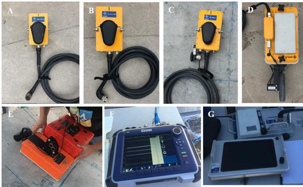
Figure 5.4 GPR equipment used in CSM Experiment (a) MALA 2.3 GHz antenna; (b) MALA 1.6 GHz antenna; (c) MALA 1.2 GHz antenna; (d) MALA 900 MHz antenna; (e) GSSI 900 (near) & 400 MHz (far) antennas; (f) GSSI SIR 4000 control unit (g) MALA control unit
