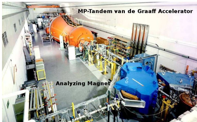
Figure 2.4: Bird's eye view of the tandem accelerator and the analyzing magnet which deflects the beam into the desired experimental hall. The beam is then sent to the target and the magnetic spectrograph. Reproduced from [7].
