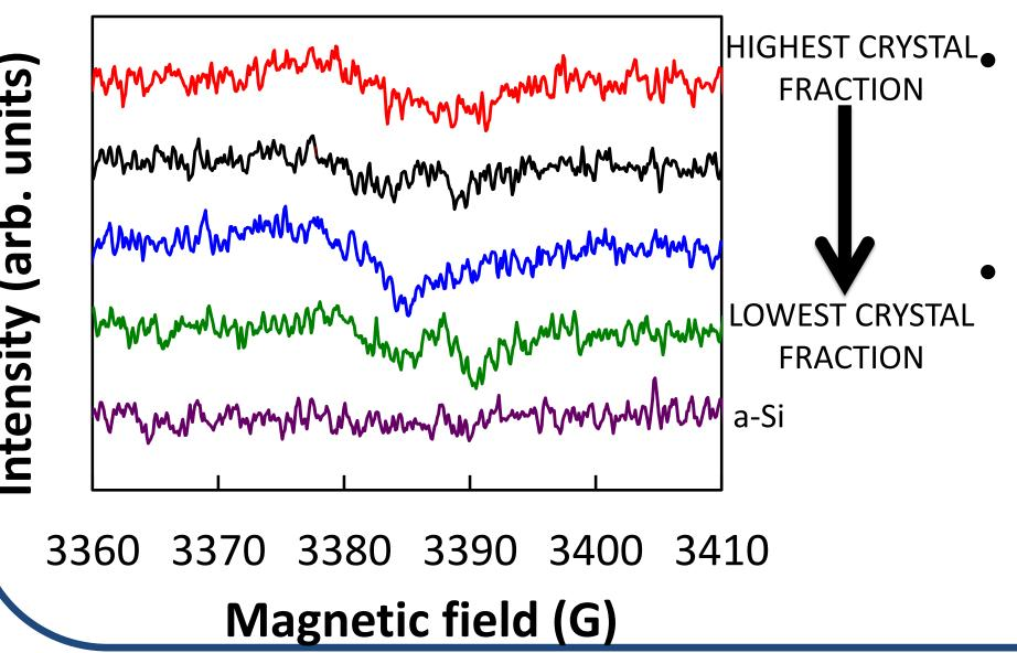
The peaks in the data shows that the materials are not defect free. Based on past results we assume the defects are probably Si dangling bonds on the surface of nanoparticles.
