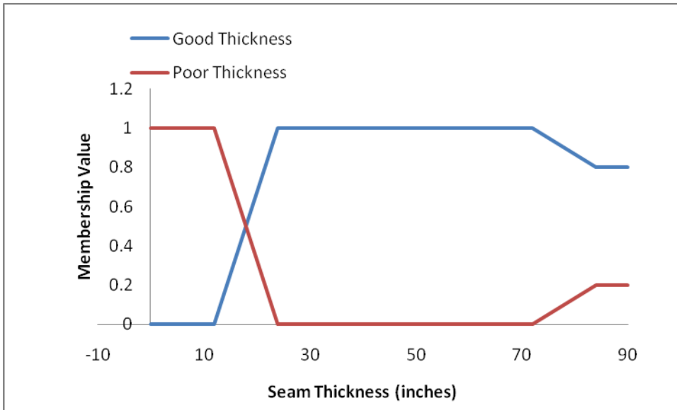
Figure A.8 Fuzzy sets for the third generation of coal cutting equipment.
