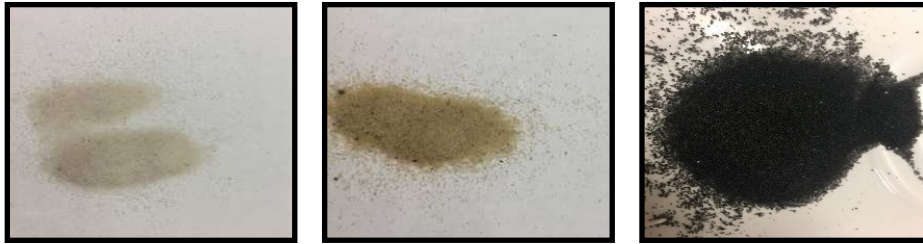
Figure 3.11: The left-hand side represents 100 mesh. The middle represents 40/70 mesh. The right-hand side represents 14/40 mesh.
