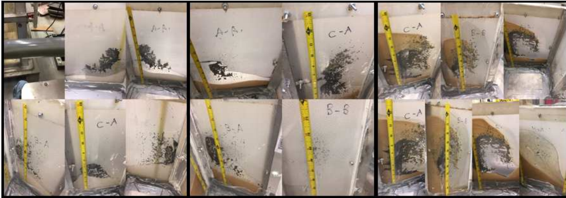
Figure 4.19: Using the water system, the blocking issue was very prominent because of the low viscosity, and the proppant particles stick to the wall of the fracture.
