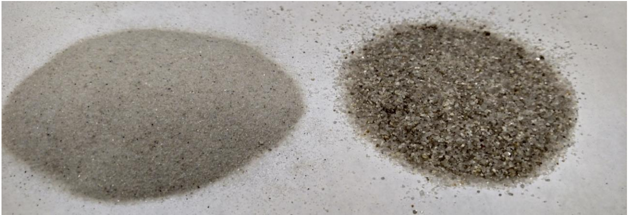
Figure 5.3 Photo of the two sand sizes tested. The fine grained sand (7030, left) and the coarser grained sand (4095, right) are pictured.
