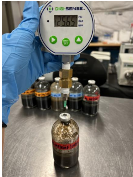
Figure 2.1 The microcosms were assembled using 160 ml bottles, a self-healing injection port, and crimp caps to allow recurrent gas pressure measurements.
