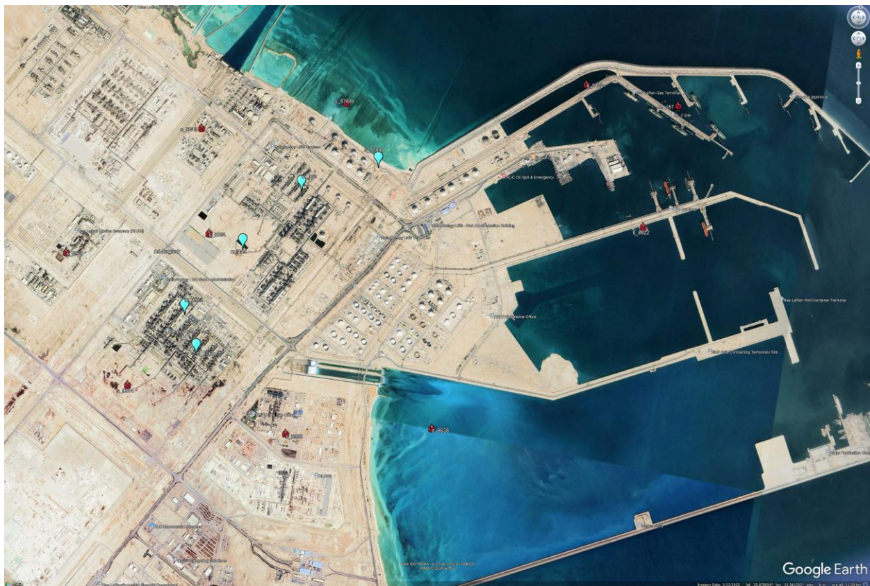
Figure 1. Map of flare locations in the Ras Laffan LNG cluster showing sites with an apparent regime change. The highlighted (cyan) sources exhibit a shift from a mixed thermal signature to one dominated by a stronger high-temperature flare component.
