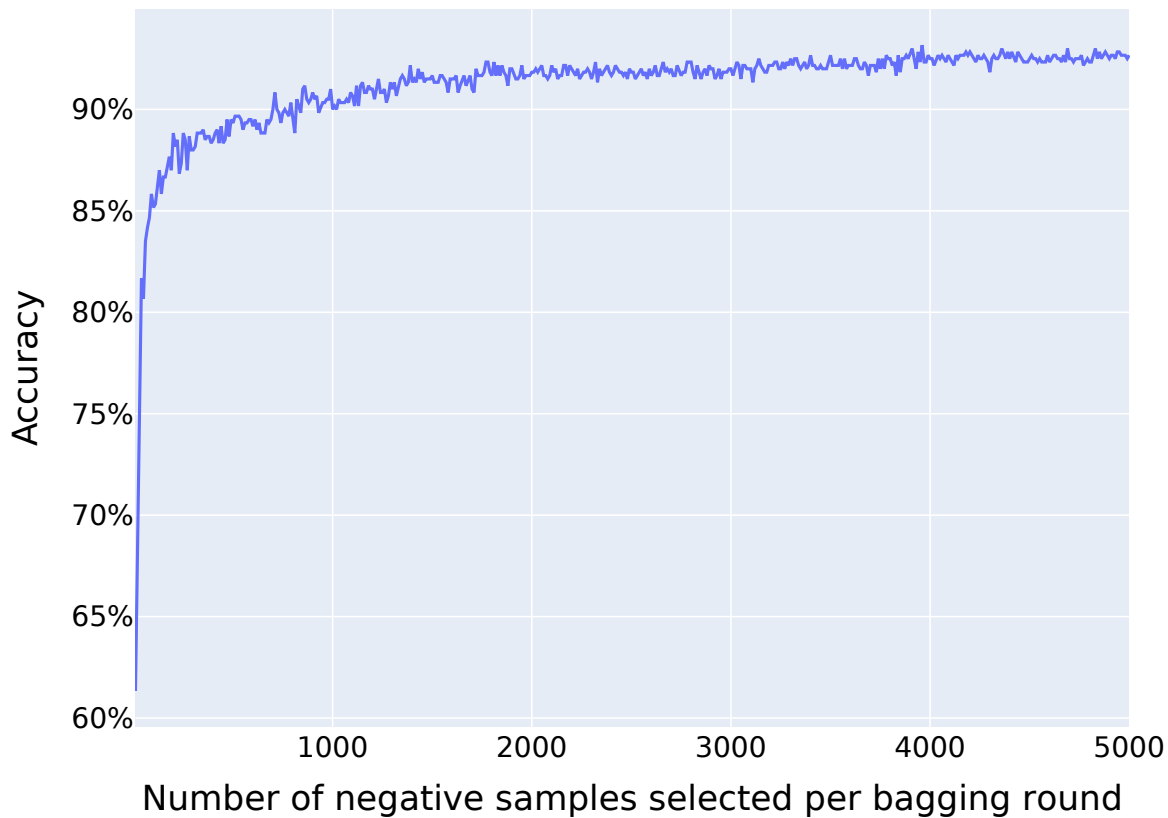
Figure 4.2 This figure illustrates the effect of changing the number of negative training samples shown to our model during bootstrap aggregation. As the number of negative training samples shown to our model increases, the accuracy obtained on classification also increases. On the lower end, at 50 negative samples, we achieve just over 81.2% accuracy. Increasing the number of negative training samples to 200 results in an improvement to 89.0% accuracy. Increasing the number of negative training samples to 5,000 results in a steady increase in accuracy, with 92.8% as the best accuracy for approximately 3,500 samples.
