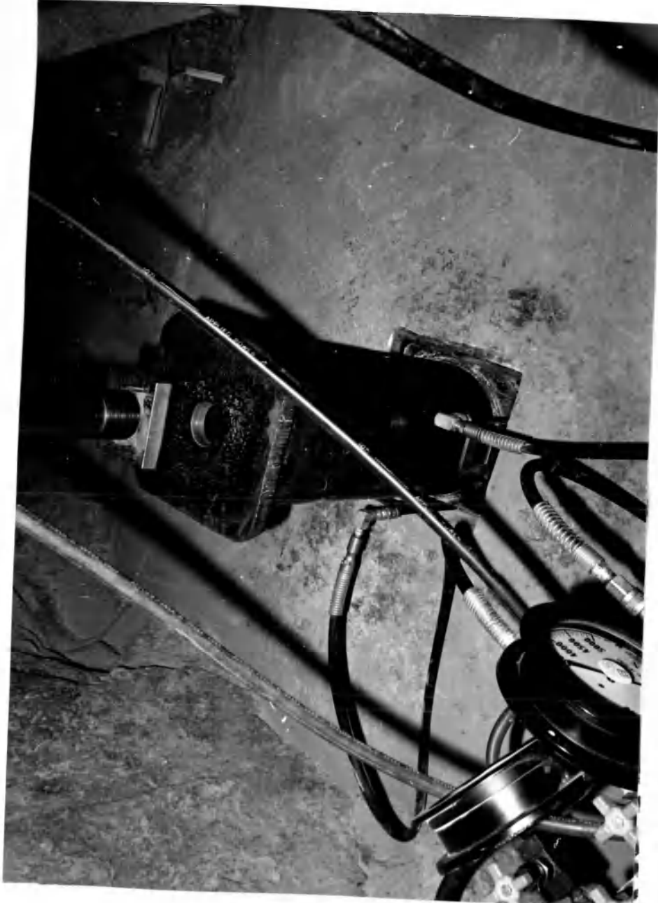
fig. A. 5 - Detail of load transfer column mounted in test hole
