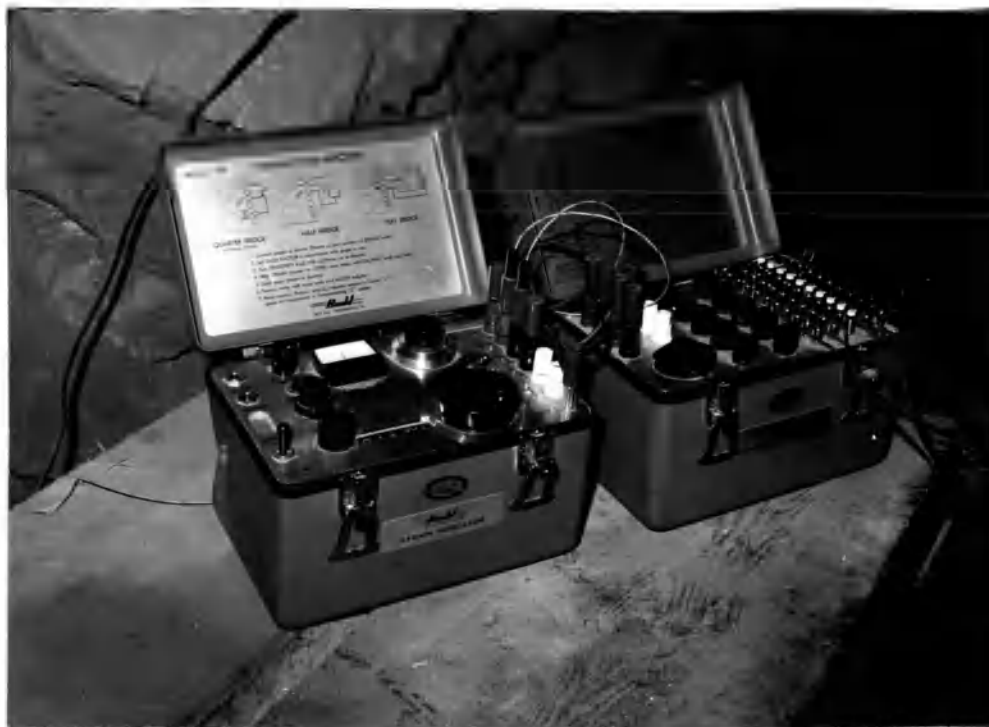
fig. A. 9 Budd strain indicator and switch and balance unit
