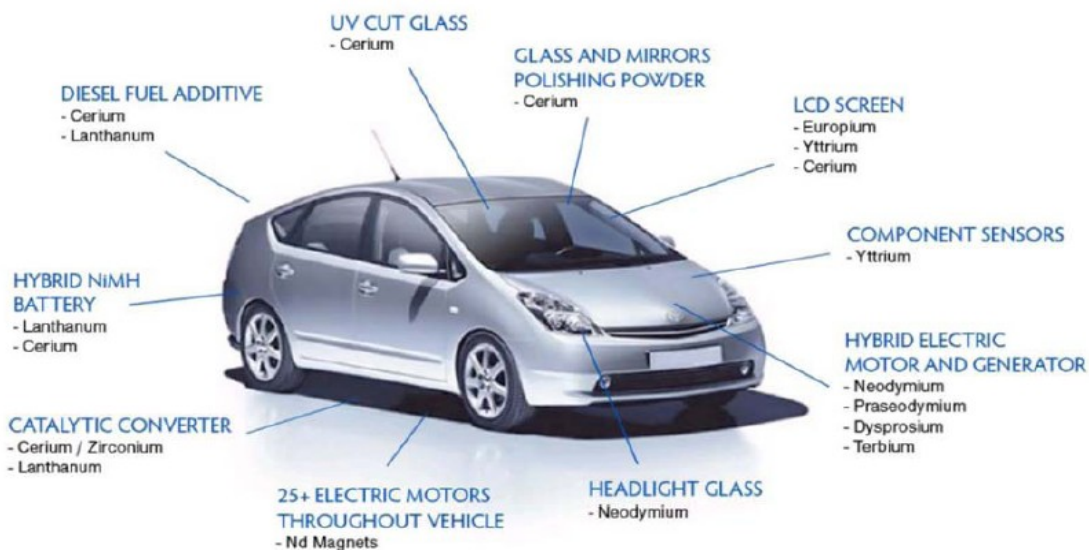
Figure 2.5 Rare earth element use in hybrid electric vehicles (Molycorp 2011).
