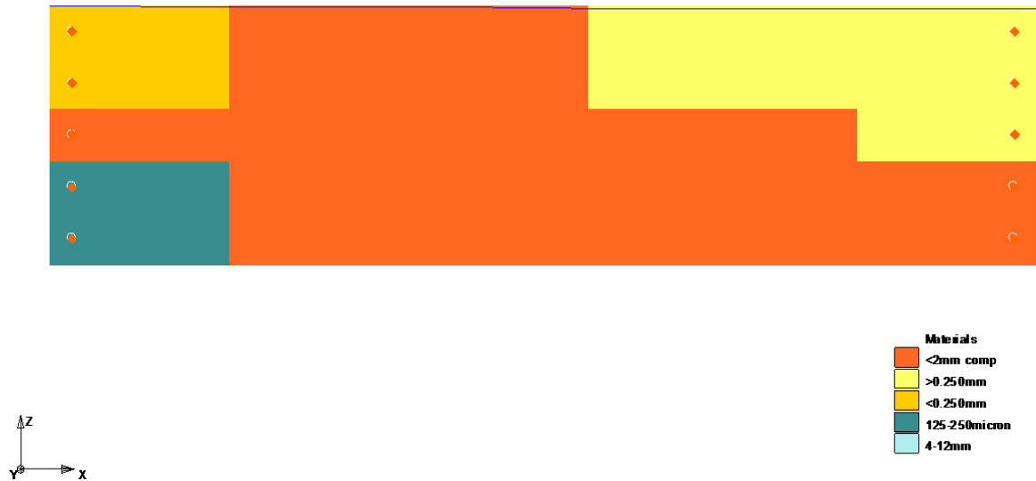
Figure 2.11 Vertical cross section of tank #3, upgradient end on the left, downgradient end on the right, y-dimension (into the place of the page) ~50.3cm (~11.2cm thick)
