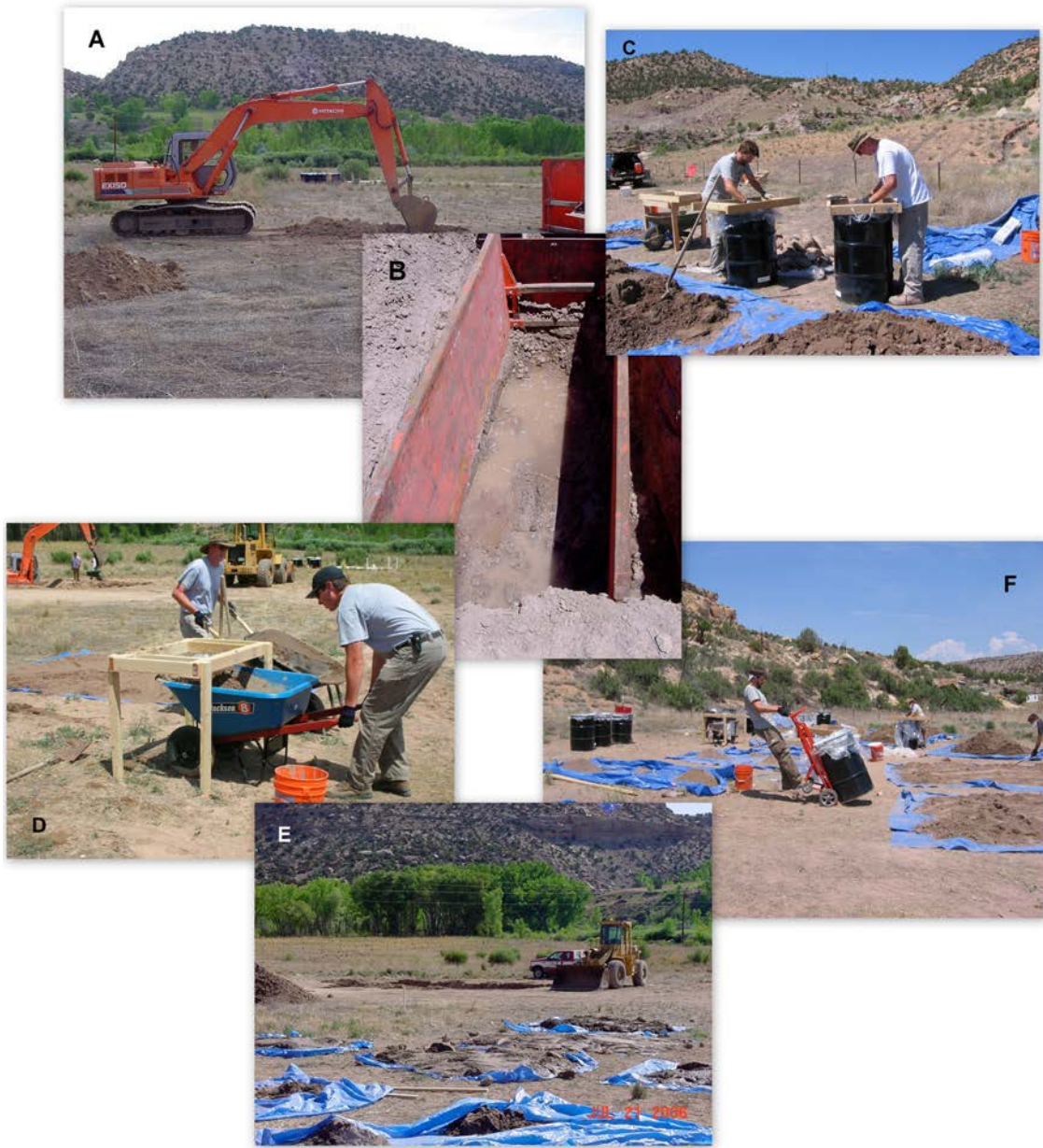
Figure 2.2 Pictures from the 'Big Dig' 2006, A- The backhoe breaks ground, B- The groundwater table is reached, the metal box maintains vertical wall integrity while digging below the water table, C- The <math><2\text{mm}</math> composite was sieved directly into the drums, D- Larger size fractions were separated in wheel barrows, E- Groundwater sediments drying in the sun, F- Once full, the drums were shipped in a moving truck back to Colorado School of Mines
