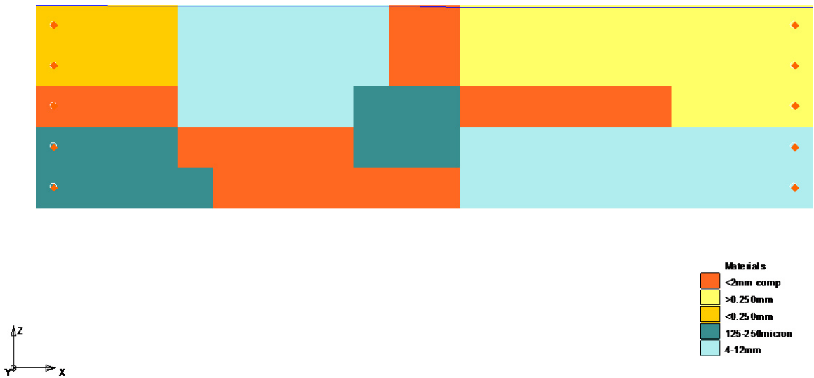
Figure 2.10 Vertical cross section of tank #3, upgradient end on the left, downgradient end on the right, y-dimension (into the plane of the page) ~39.1cm (~11.2cm thick)
