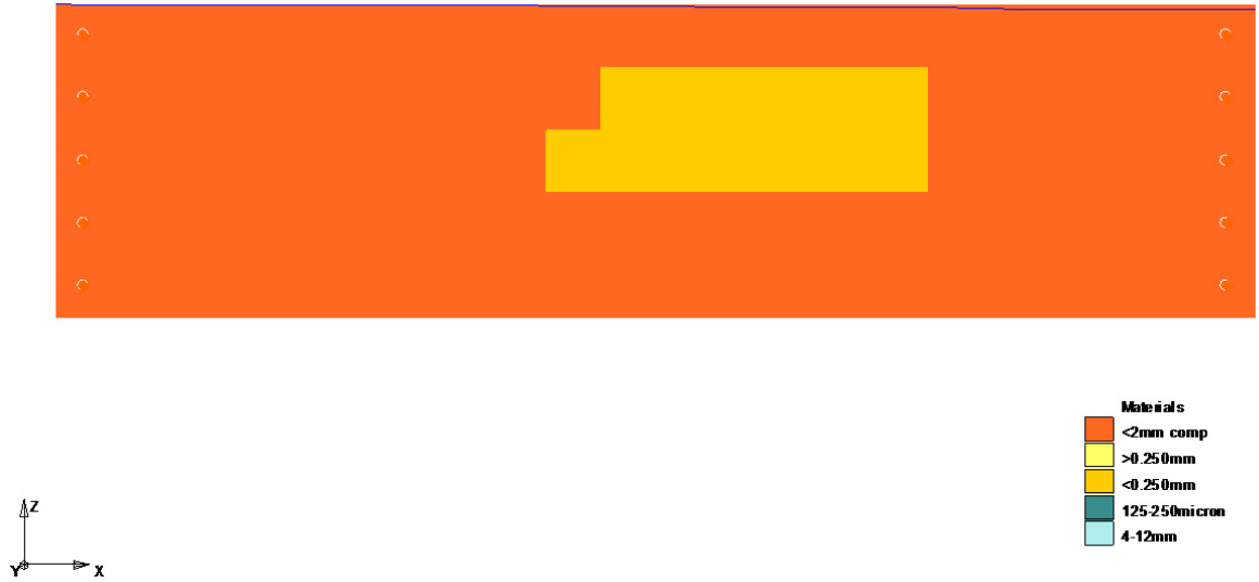
Figure 2.7 Vertical cross section of tank #3 packing, upgradient end on the left, downgradient end on the right, y-dimension (into plane of page) ~5.6cm (~11.2cm thick)
