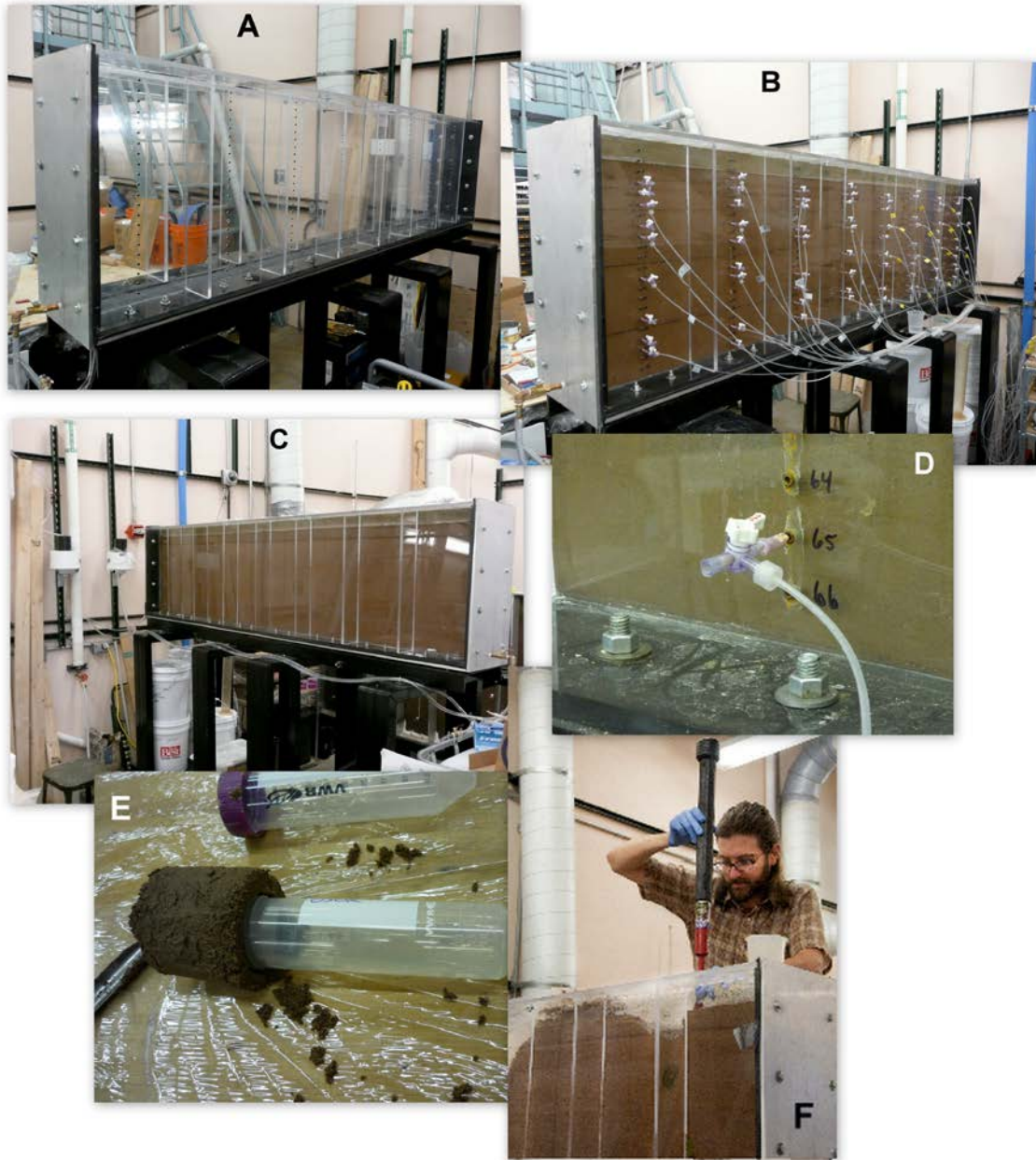
Figure 2.3 Construction and packing of tank #2, A- Fully constructed tank #2, gasket material clearly visible in black, B- Tank #2 fully packed, saturated and connected to pressure array, C- Opposite view as B, head boundaries in background, D- 3-way valve in sampling port connected to pressure array, E- Taking a core of the core for microbial analysis, F- Taking a core from the tank
