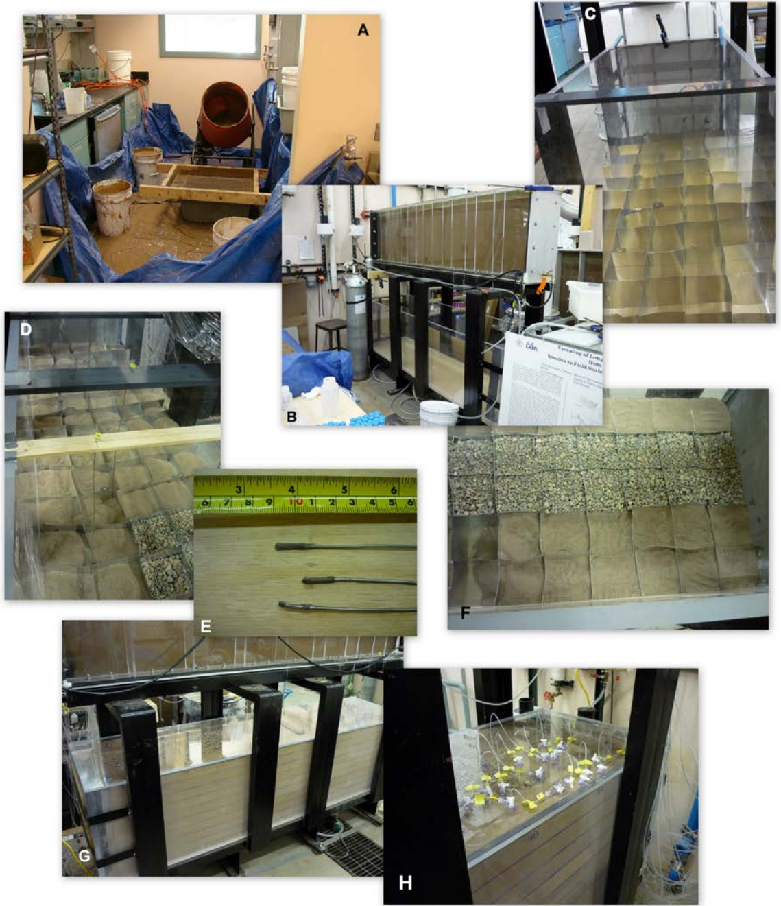
Figure 2.6 Tank construction and packing of tank #3, A- Wet sieving of 4-12mm size fraction, B- Tank #3 fully constructed underneath tank #2, C- Aluminum grid in place creating ~11cm cubes, D- Packing of the various size fraction in the aluminum grid with several sampling wells in place, E- The screened end of the sampling wells, F- Packing of the various size fractions, G- The tank is fully packed, and the lid is in place and caulked, H- Sample tubing and three way valves connected to the sampling wells.
