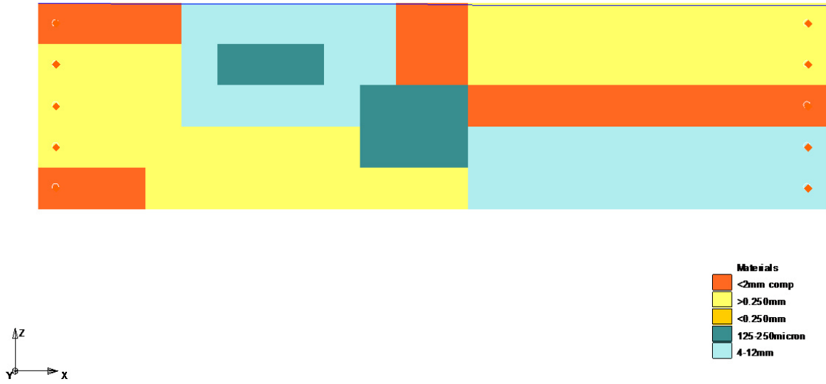
Figure 2.9 Vertical cross section of tank #3, upgradient end on the left, downgradient end on the right, y-dimension (into the plane of the page) ~28.0cm (~11.2cm thick)
