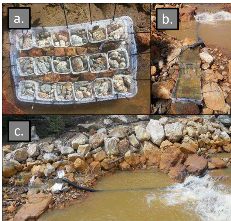
Figure 4.2: Pictures of the side-of-the-stream deployment method at Site 2. (a) The field-mesocosm bin holding 18 rock trays, with stream rocks placed in between the trays for additional weight; (b&c) the stream-side deployment showing the placement of the irrigation tube and holding bins.
