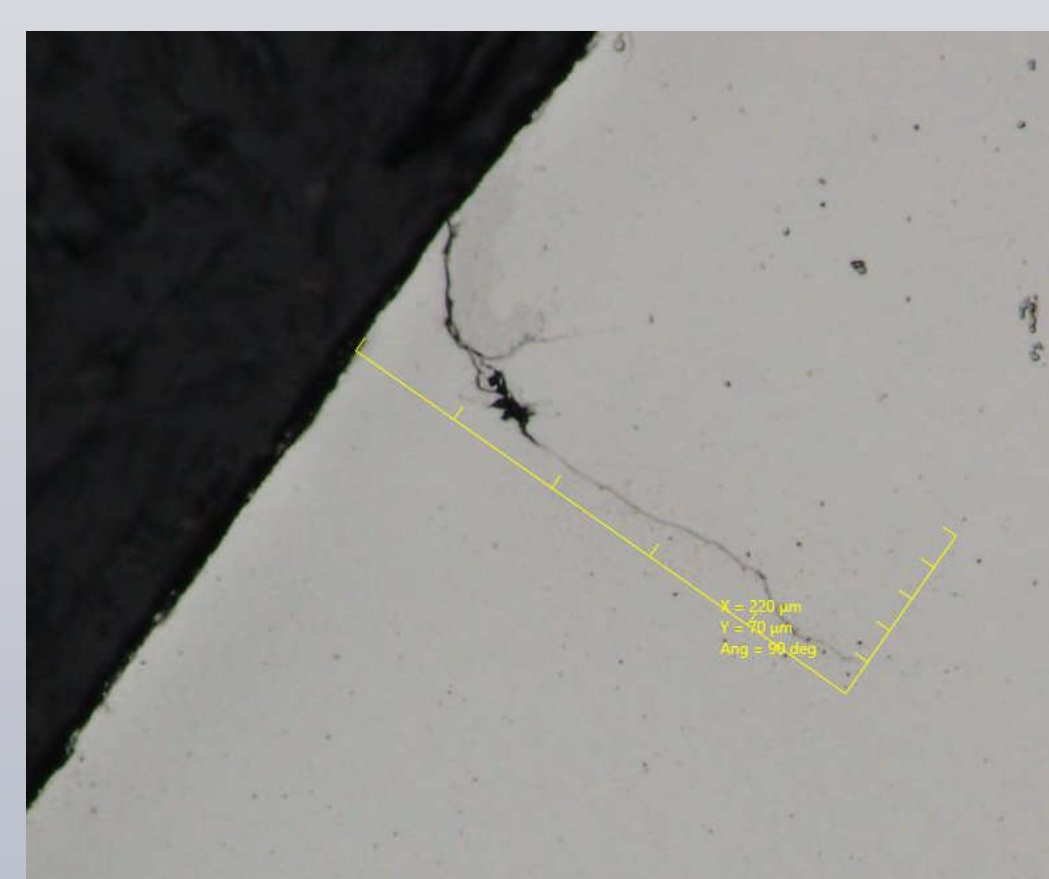
Figure 5: 0.009" deep crack in nanostructured Titanium annealed at 375°C
