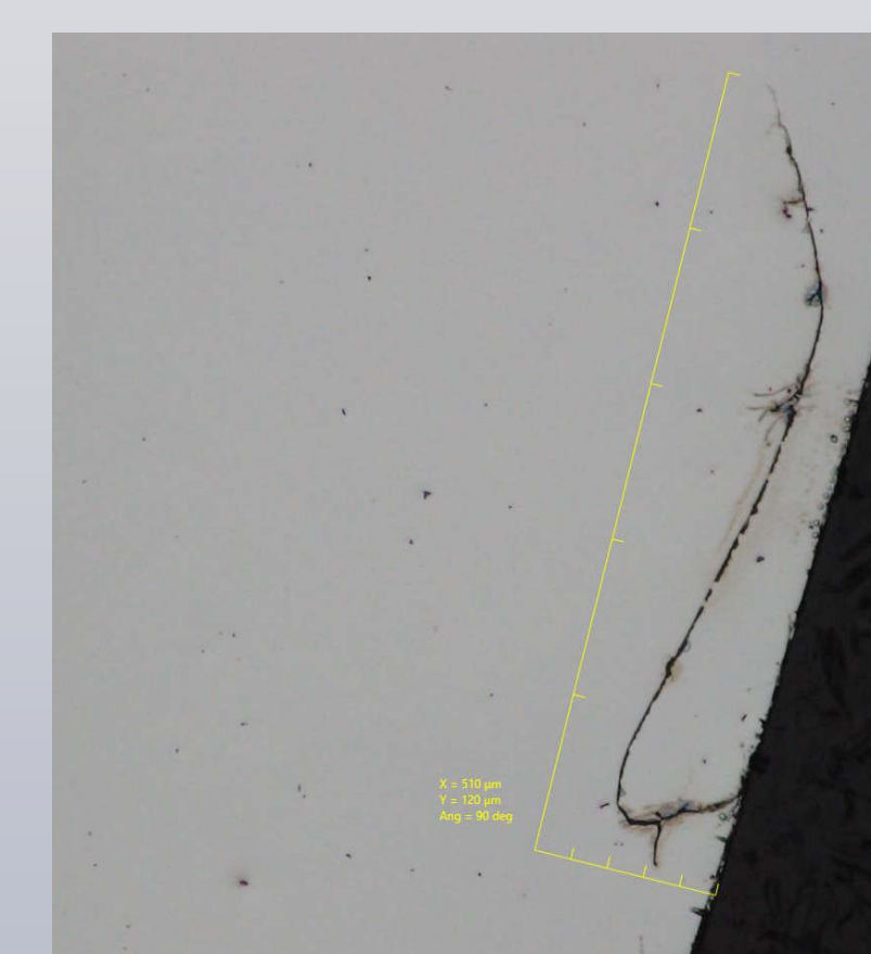
Figure 6: 0.005" deep crack in nanostructured Titanium annealed at 300°C
