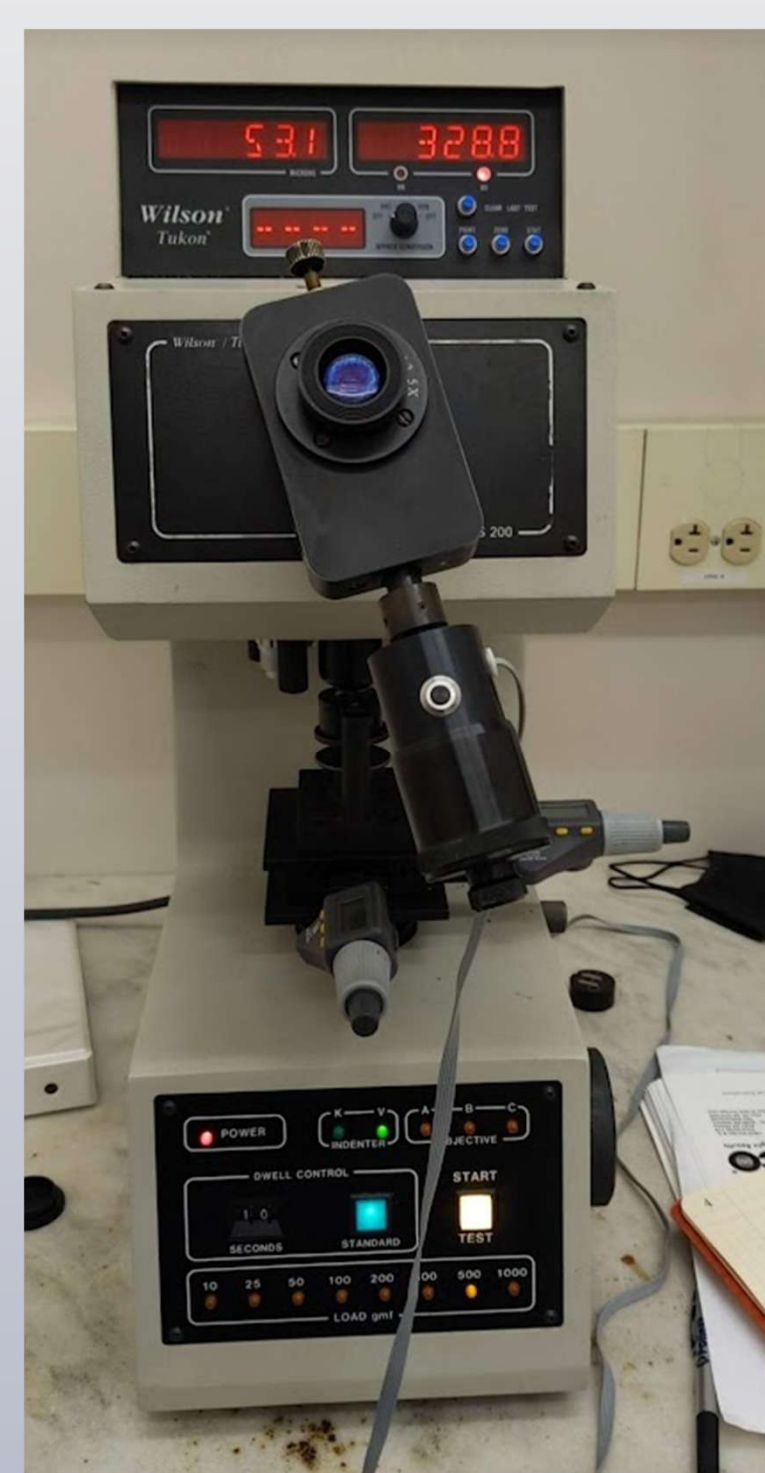
Figure 3: Manual Vickers Microhardness Indenter
