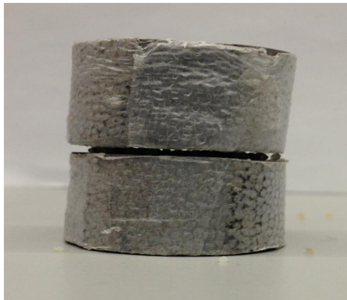
Figure 4.26: Image of proppant loading setup. Proppants are placed in between bottom and top cores.
