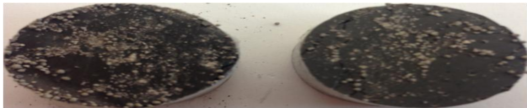
Figure 5.39: Bottom and top cores from KCl+friction reducer Test#1 loaded with 20/40 Brady at 0.1 lb/ft 2 after they were subjected 3030 psi for one hour. Core diameters are 1.0 inch.
