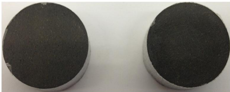
Figure 4.30: Images of bottom (left) and top (right) cores from Freshwater Test#2 without any pressure or proppant effect. Core diameters are 1.0 inch.
