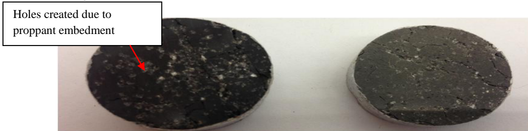
Figure 4.35: Bottom and top cores from Freshwater Test#1 (pressured to 3030 psi for 1 hour) after 16/30 Brady proppants are removed. Core diameters are 1.0 inch.
