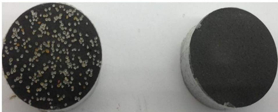
Figure 4.32: Bottom and top cores from Freshwater Test#2 loaded with 20/40 Ottawa at 0.1 lb/ft 2 (no pressure). Core diameters are 1.0 inch.
