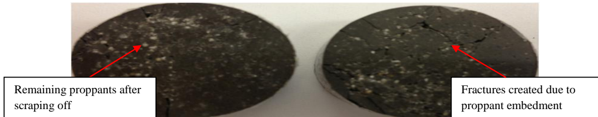
Figure 4.36: Bottom and top cores from Freshwater Test#2 (pressured to 3030 psi for 1 hour) after 20/40 Ottawa proppants are removed. Core diameters are 1.0 inch.
