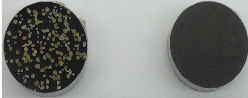
Figure 4.31: Bottom and top cores from Freshwater Test#1 loaded with 16/30 Brady at 0.1 lb/ft 2 (no pressure). Core diameters are 1.0 inch.
