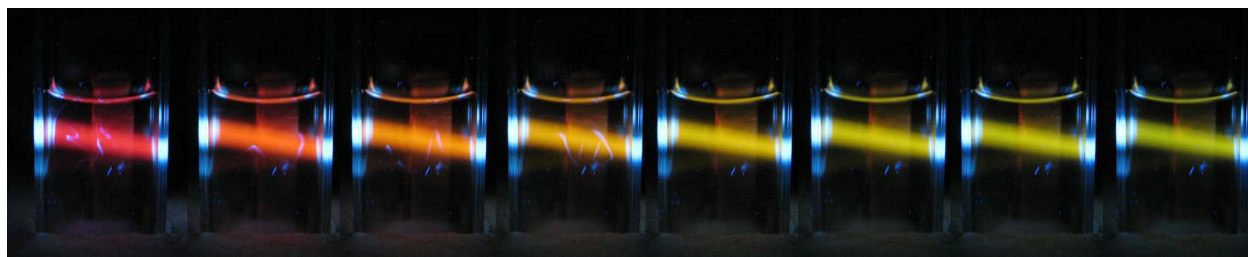
Figure 3.4: Change of luminescence color during etching. Images were taken during in-situ etching over a period of 15 minutes. The luminescing region is defined by the excitation beam passing through solution.
