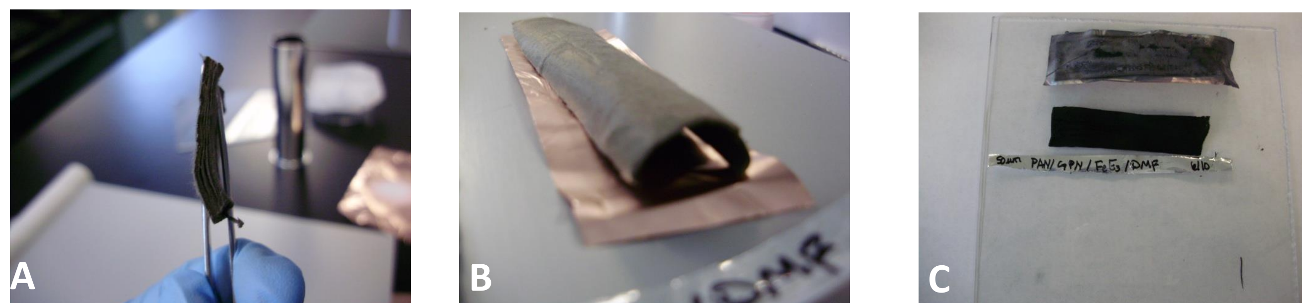
Figure 2- (A,B) Free-standing membranes of PAN/Graphene/FeE 3 . (C) Annealed intact membrane (500C for 3 hours)
