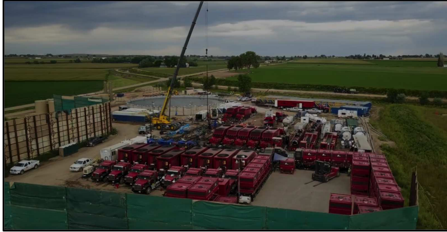
Figure 4.6: Example of a fracturing crew at an oil field completion site(Courtesy of Liberty Oilfield Services)
