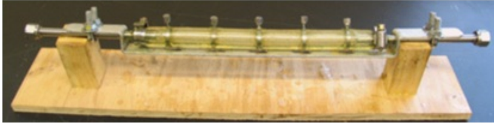
Figure 3.3: Proppant pack showing different pressure measurement points used at CSM
