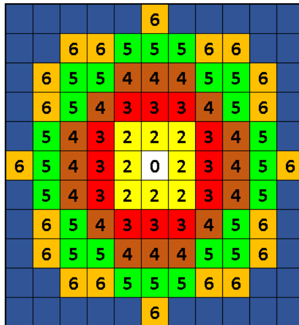
Figure A.7: Final cone pattern template for 40° pit slope angle, 50x50x35ft blocks
