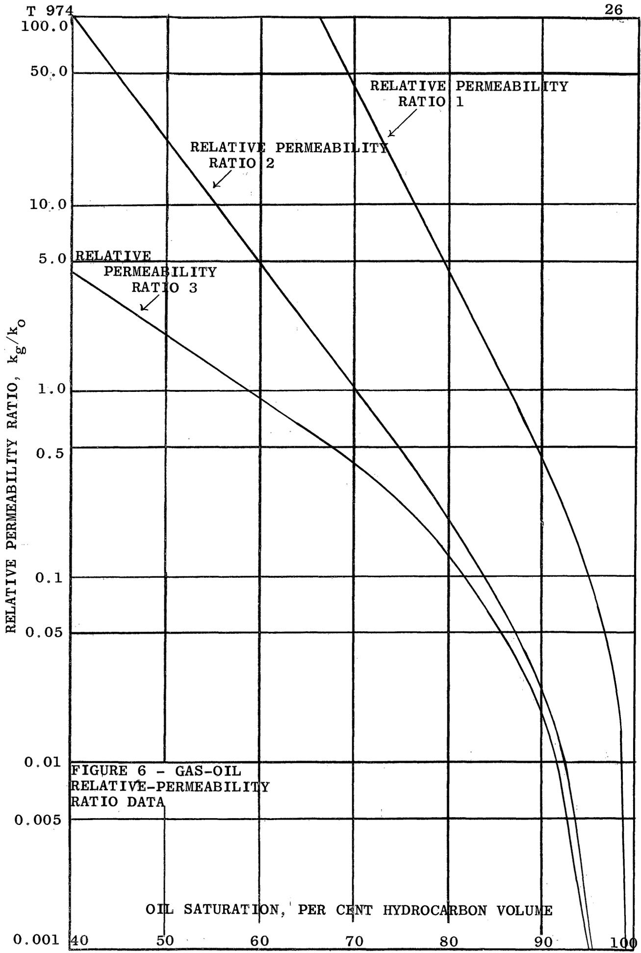
chert. Ratio 2 represents their average curve corrected for a connate-water saturation of 15 percent and is probably representative of the vugular types of limestone. Ratio 3, the most favorable, was designed to represent a consolidated sand or sandstone.
