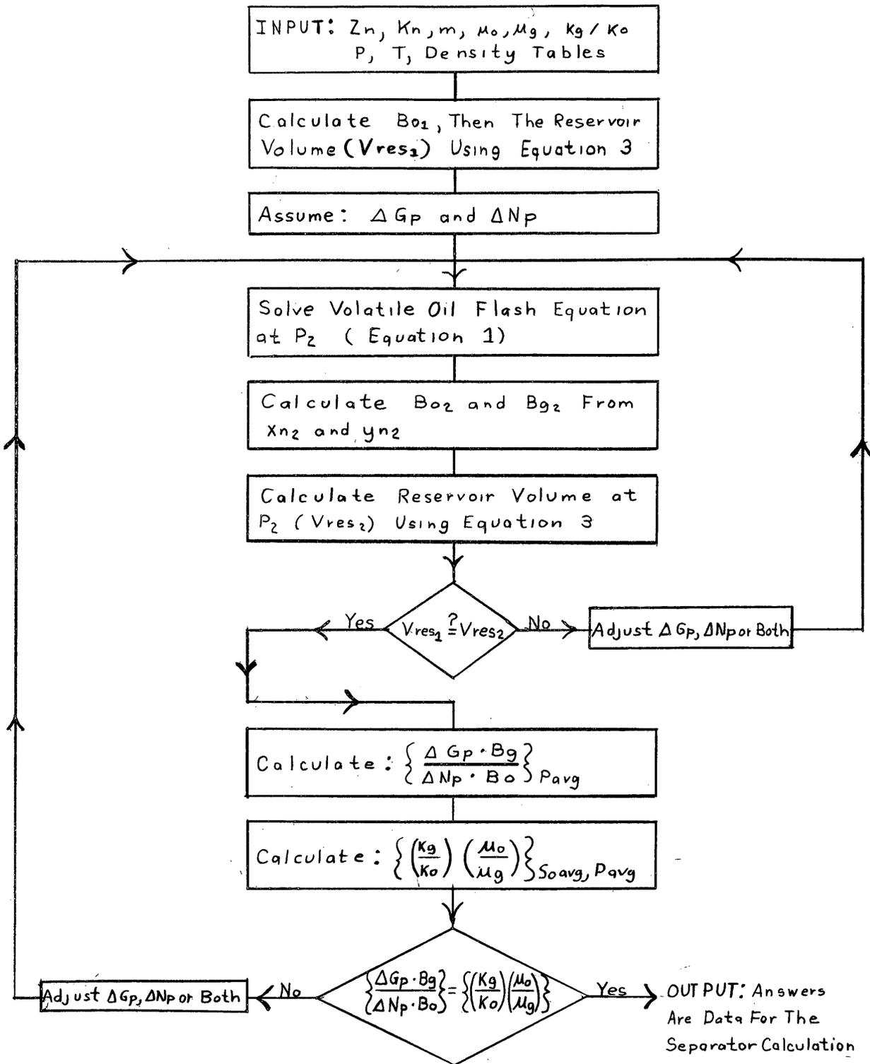
FIGURE 1 - FLOW DIAGRAM OF THE PERFORMANCE-PREDICTION METHOD
