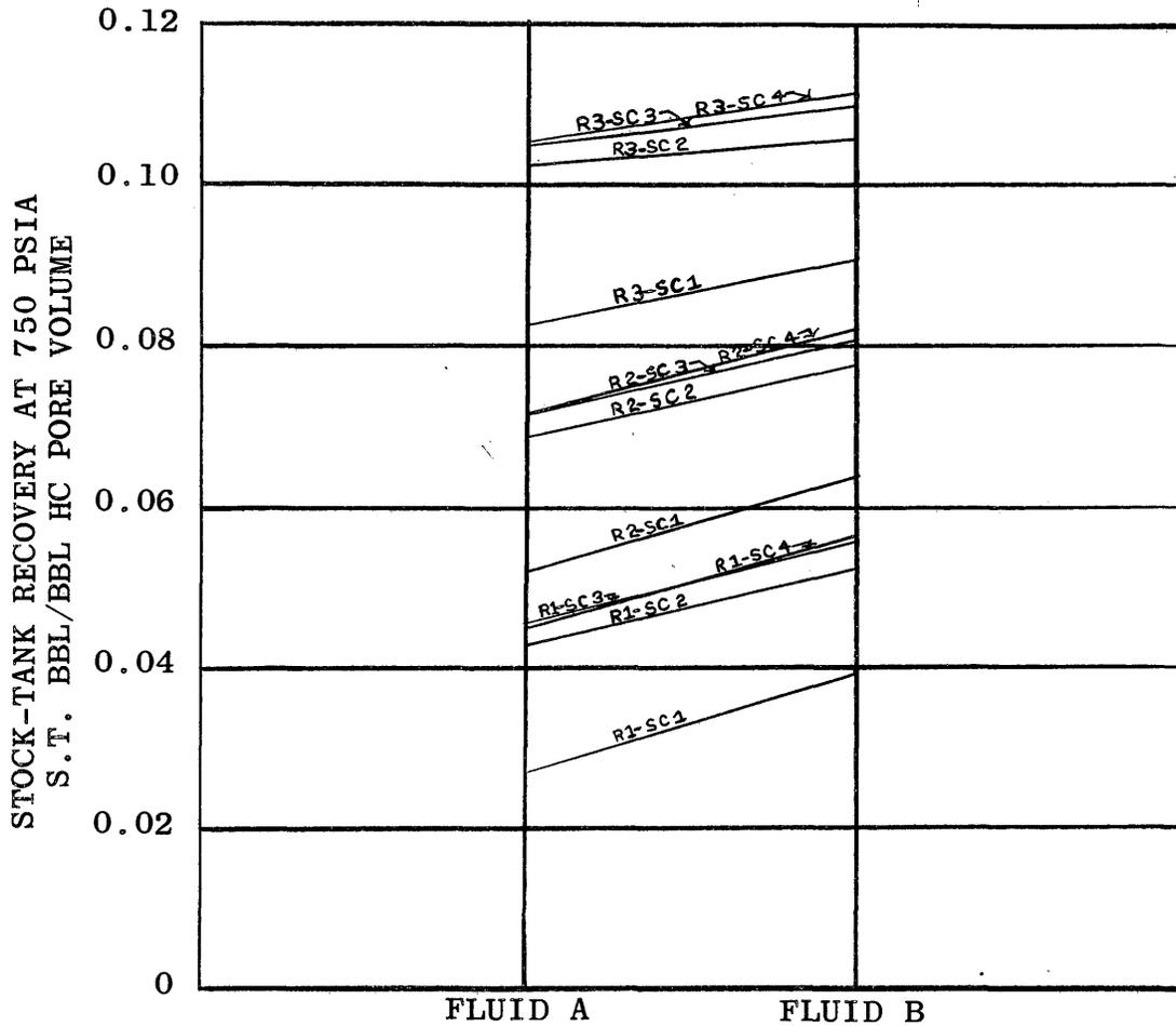
FIGURE 13 - EFFECT OF FLUID COMPOSITION ON RECOVERY AS A FUNCTION OF RELATIVE-PERMEABILITY RATIO AND SURFACE-SEPARATION CONDITIONS
