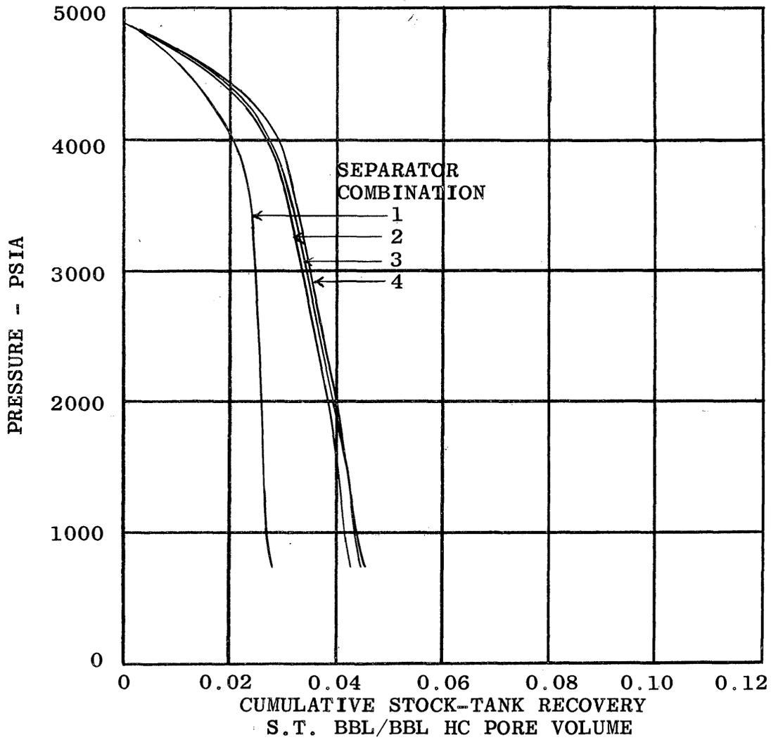
FIGURE 7 - EFFECT OF SURFACE-SEPARATION CONDITIONS ON OIL RECOVERY FOR FLUID A, AND RELATIVE-PERMEABILITY RATIO 1
