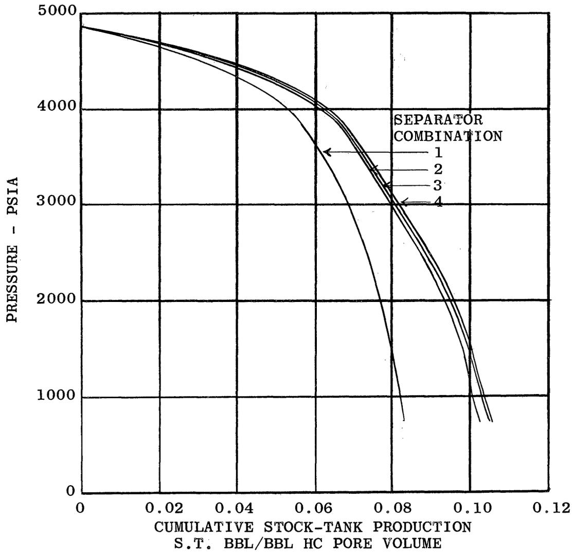
FIGURE 9 - EFFECT OF SURFACE-SEPARATION CONDITIONS ON OIL RECOVERY FOR FLUID A, AND RELATIVE-PERMEABILITY RATIO 3
