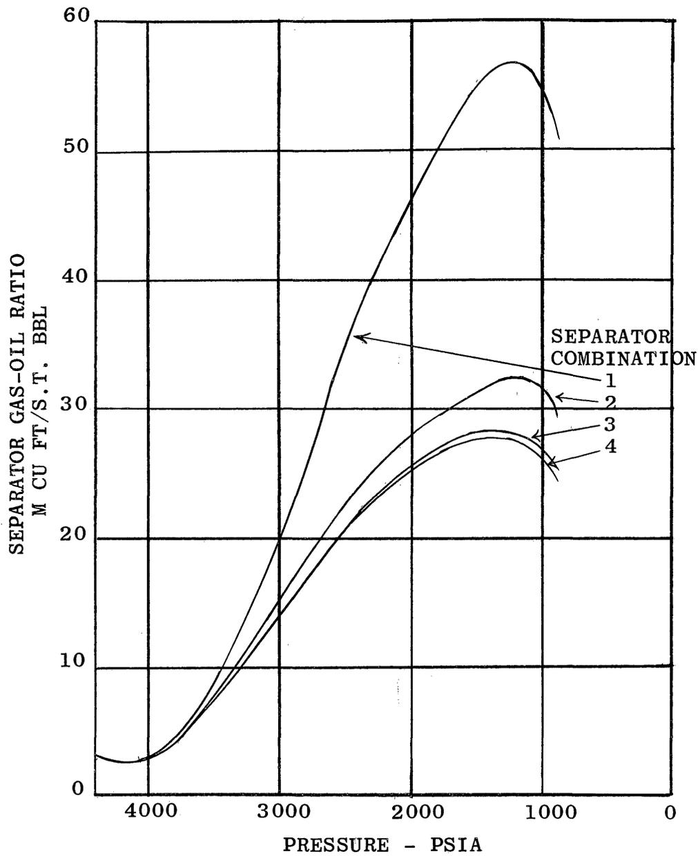
FIGURE 16 - EFFECT OF SURFACE-SEPARATION CONDITIONS ON SEPARATOR GAS-OIL RATIO PERFORMANCE FOR FLUID B, AND RELATIVE-PERMEABILITY RATIO 2
