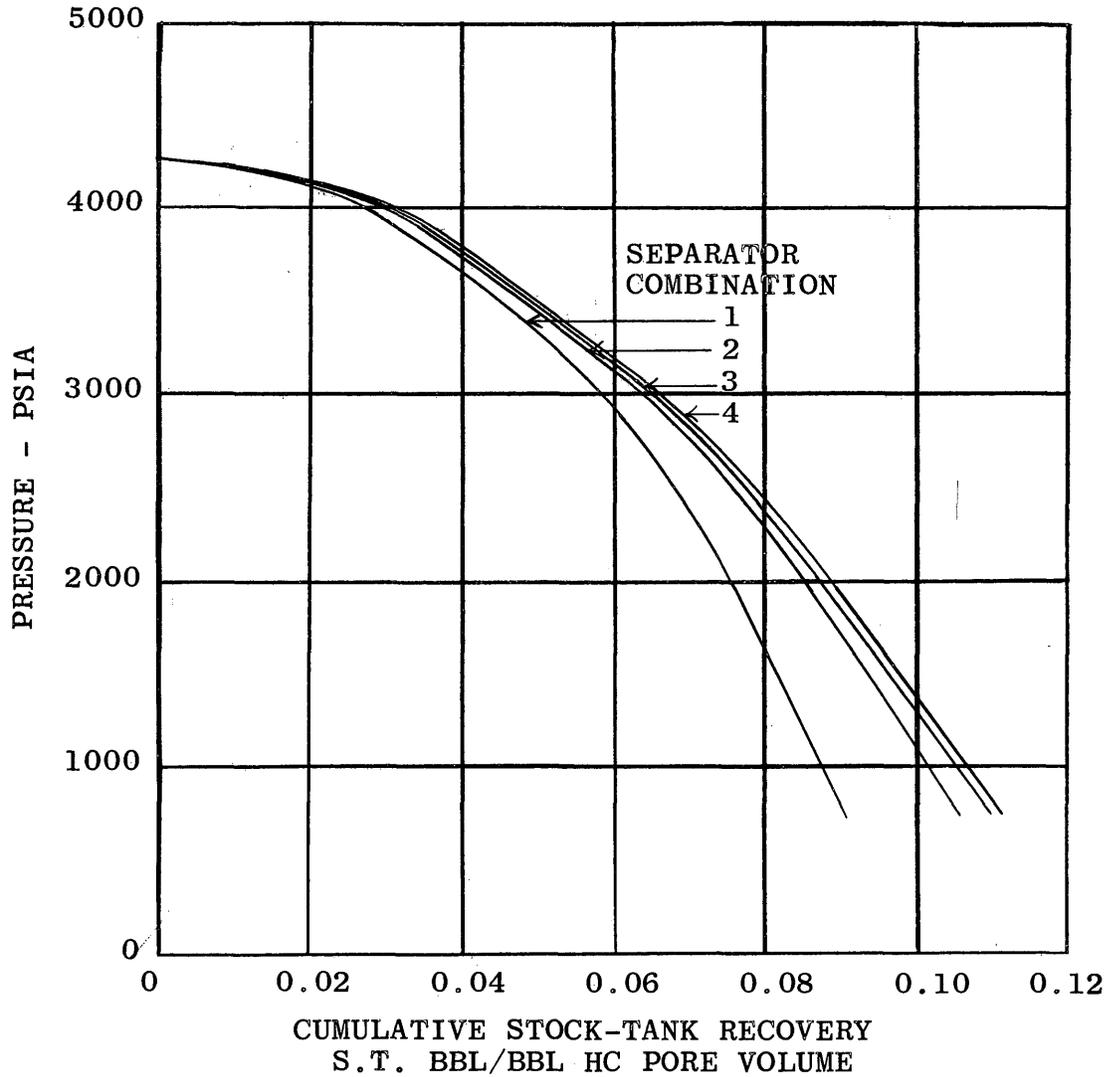
FIGURE 12 - EFFECT OF SURFACE-SEPARATION CONDITIONS ON OIL RECOVERY FOR FLUID B, AND RELATIVE-PERMEABILITY RATIO 3
