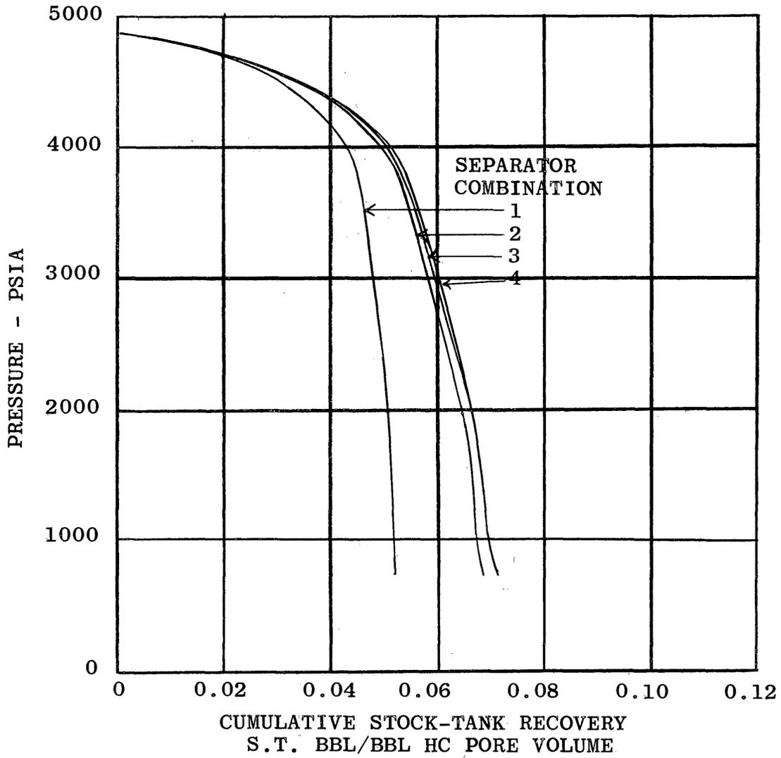
FIGURE 8 - EFFECT OF SURFACE-SEPARATION CONDITIONS ON OIL RECOVERY FOR FLUID A, AND RELATIVE-PERMEABILITY RATIO 2
