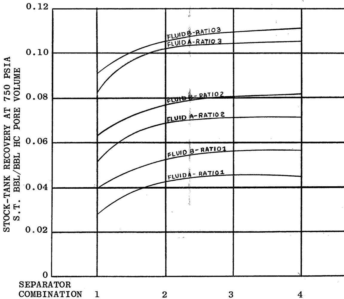
FIGURE 15 - EFFECT OF SURFACE-SEPARATION CONDITIONS ON RECOVERY AS A FUNCTION OF FLUID COMPOSITION AND RELATIVE-PERMEABILITY RATIO
