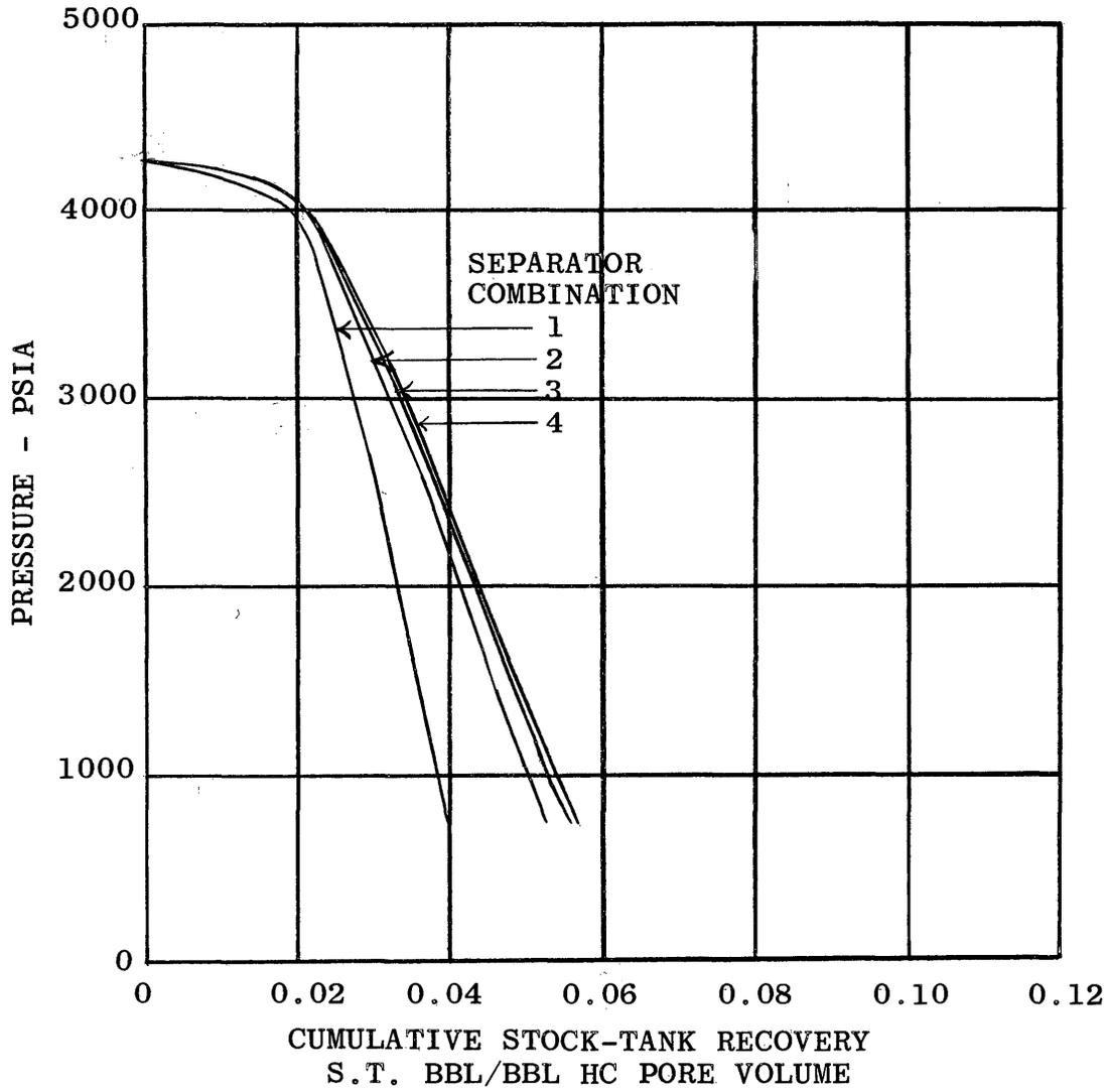
FIGURE 10 - EFFECT OF SURFACE-SEPARATION CONDITIONS ON OIL RECOVERY FOR FLUID B, AND RELATIVE-PERMEABILITY RATIO 1
