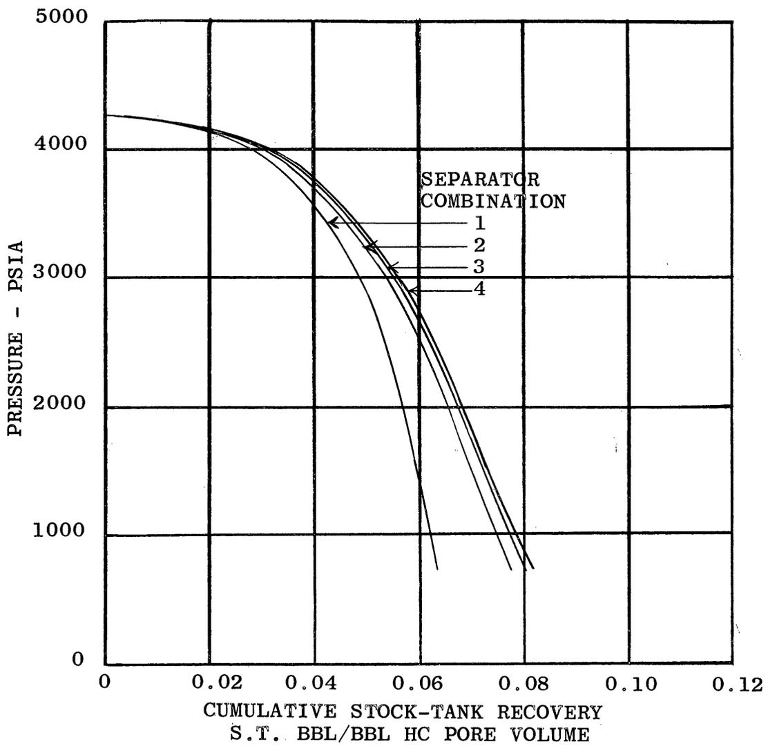
FIGURE 11 - EFFECT OF SURFACE-SEPARATION CONDITIONS ON OIL RECOVERY FOR FLUID B, AND RELATIVE-PERMEABILITY RATIO 2
