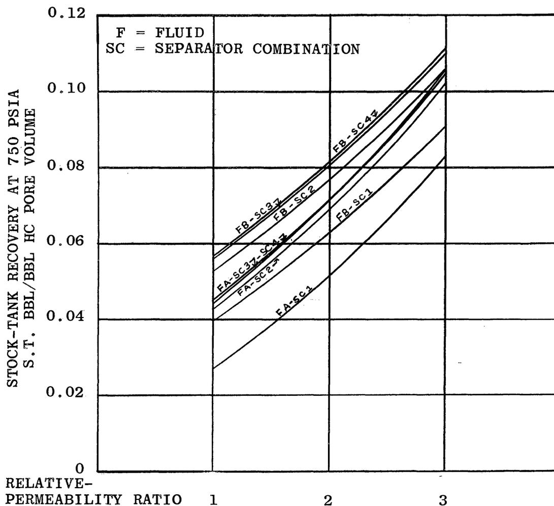
FIGURE 14 - EFFECT OF RELATIVE-PERMEABILITY RATIO ON RECOVERY AS A FUNCTION OF FLUID COMPOSITION AND SURFACE-SEPARATION CONDITIONS
