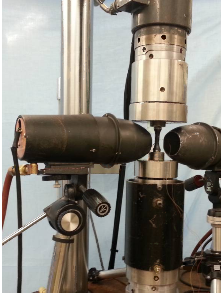
Figure 3.6 The 100 kip MTS servo-hydraulic frame with woodmetal alignable grips and heat lamps in place for elevated temperature Bauschinger effect testing. The matte black paint to improve heating from the lamps is visible on the surface of the sample as well as the thermocouple wires from the spot welded k-type thermocouple for temperature control.
