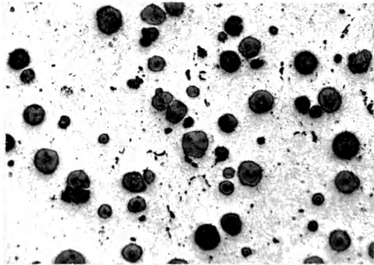
Figure 17. Mg-Ni nodular cast iron, Soaked at 1600 F for 8 hours, Water quenched, Etched 40 seconds with 2% nital. Magnified 100X
