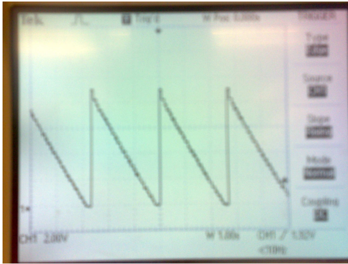
Figure 8.6: V_{out} versus time as obtained from the oscilloscope.
