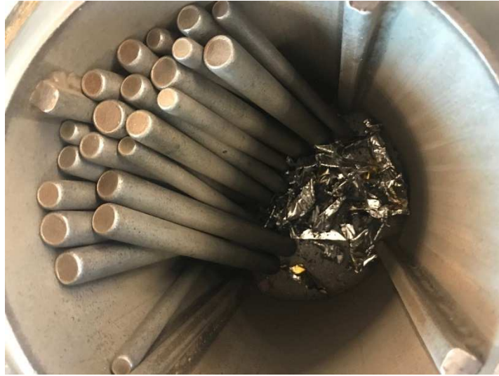
Figure 3.2: Rod mill with rod charge and non-ferrous material charge.
