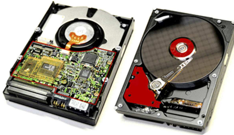
Figure 2.8: left: computer hard drive. Right: Hard drive with the back plate removed to reveal the internals. The red shaded regions indicate the assemblies containing magnet material.
