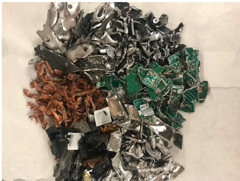
Figure 3.20: Sorted metals from shredded hard drive.
