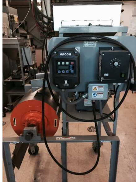
Figure 3.5: Eriez Rare Earth 15 inch drum.
