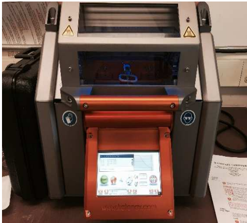
Figure 3.17: Fuser used for preparation of fused samples.
