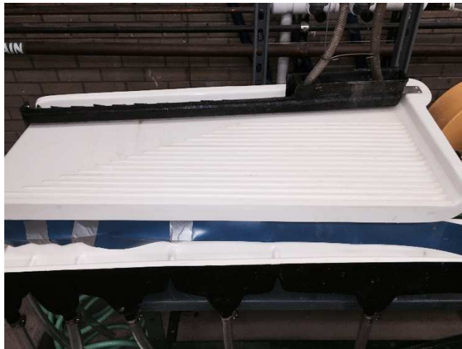
Figure 3.10: Shaking Table. The heavy fraction comes off the left side of the table, The light fraction comes off the right side over the ridges.
