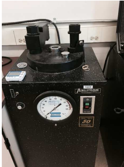
Figure 3.16: Press used to prepare XRF samples.
