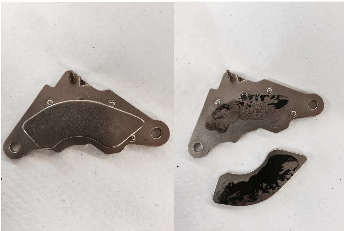
Figure 3.4: image of magnet assembly before and after demagnetization
