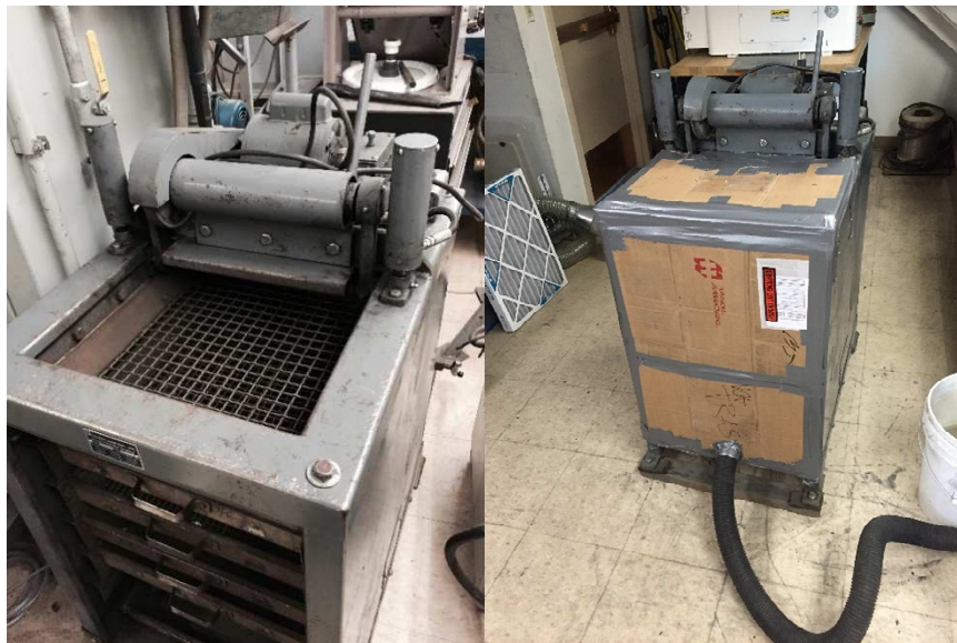
Figure 3.12: Gilson screen (left) with screens installed. Dust cover installed (right) with air draw to bag house visible at bottom of the image.
