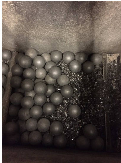
Figure 3.3: Ball mill with shredded hard drive and ball charge.
