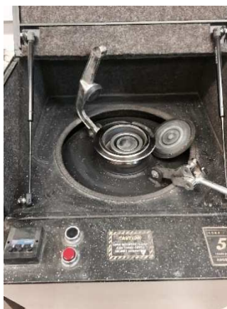
Figure 3.15: Pulverizer for fine grinding of XRF samples.
