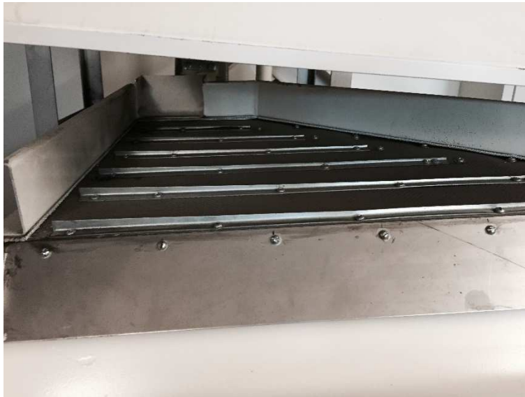
Figure 3.11: Air table density separation equipment
