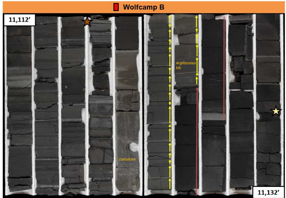
Figure 2.8—Wolfcamp B facies distribution and example of cored interval spanning 20 ft. The core depth, facies group, and lithofacies can be found on the left. Pie charts of the facies group and lithofacies distributions are seen below. The red box is the cored example shown. An example of one carbonate sediment gravity flow deposit is shown in the red arrow. Yellow arrows represent individual fine-grained turbidites associated with the argillaceous mudstone lithofacies. The brown star shows RCA location for argillaceous mudstone at 11,118 ft (LECO TOC 0.81 wt.%, porosity 10.0%, permeability 1.63 nD, and water saturation 74.9%). The yellow star shows RCA location for siliceous mudstone at 11,131 ft (LECO TOC 2.33 wt.%, porosity 9.3%, permeability 52.5 nD, and water saturation 55.5%).
