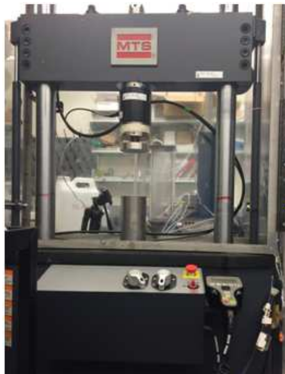
Figure 3.8: MTS load apparatus used for uniaxial testing.
