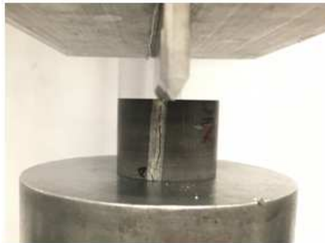
Figure 3.11: Brazilian tensile tests conducted to obtain naturally rough fracture surfaces for the triaxial stress state measurements.
