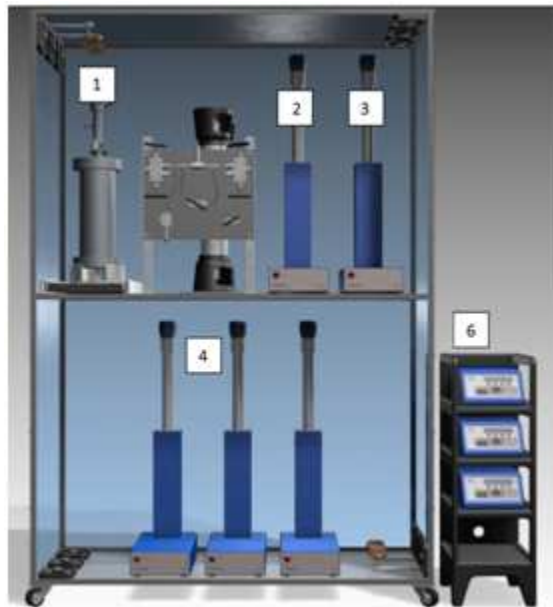
Figure 3.16: 3D view of the components of the triaxial stress experimental setup (Padín 2016).
