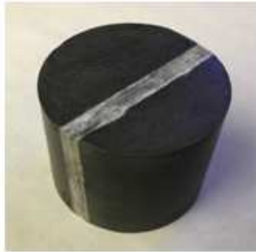
Figure 3.10: Niobrara outcrop core plug containing a thick calcite-filled fracture (Nio-2.1) used for the triaxial stress test.
