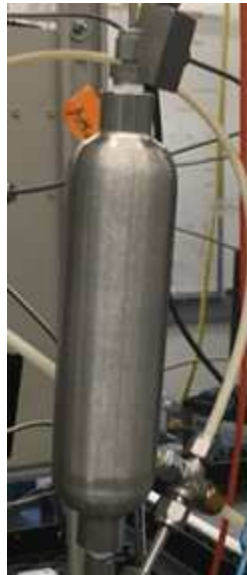
Figure 3.25: Sampler used to collect fluid from the triaxial stress experimental setup.
