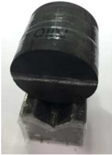
Figure 3.15: Fracture core filled with a proppant monolayer and wrapped with tape around the circumference.
