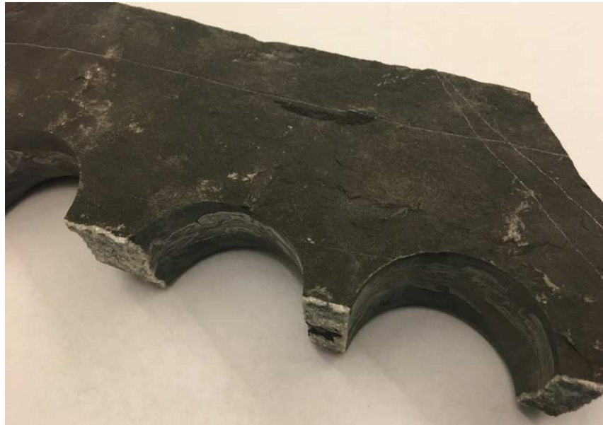
Figure 3.12: Niobrara outcrop block failed in the main calcite-filled fracture (weakest plane in the sample) and the presence of microfractures.
