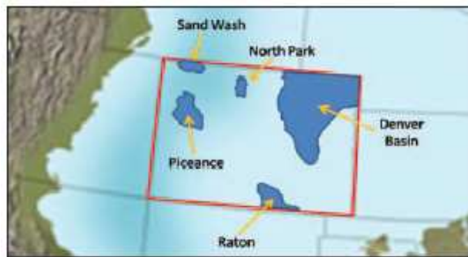
Figure 1.3: Basins (dark blue) with known shale oil potential overlaid on paleogeographic map of Late Cretaceous (Matthews 2011).
