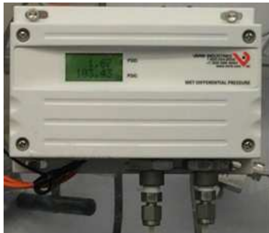
Figure 3.24: Veris PWLX05S wet Pressure Differential Transducer.
