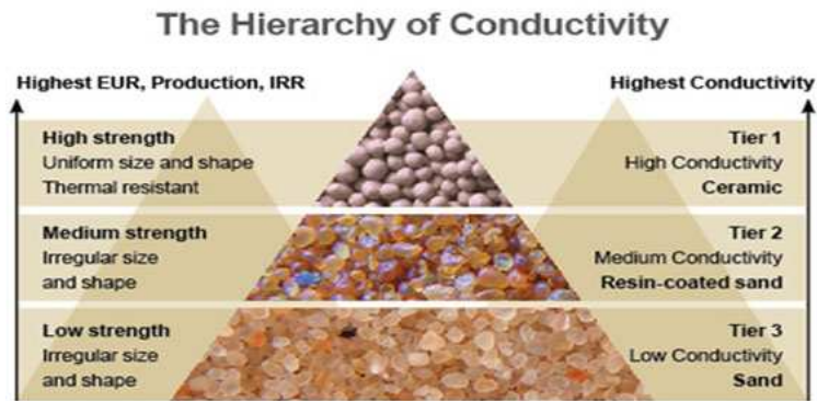
Figure 2.4: Different proppant types and their classification according to their strength and conductivity (Kullman 2011).
