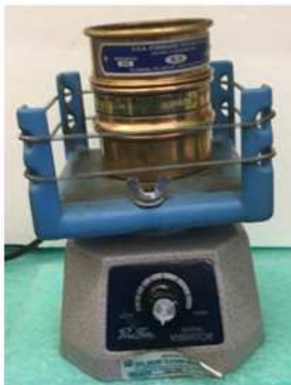
Figure 3.13: Proppant sieve on a dental vibrator to separate the 40-mesh grains size.
