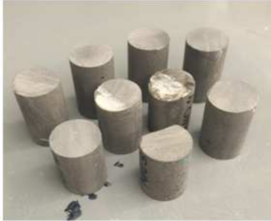
Figure 3.3: Niobrara outcrop core plugs used for the geomechanical variations test saturation process proceeded at room temperature for 30 days.
