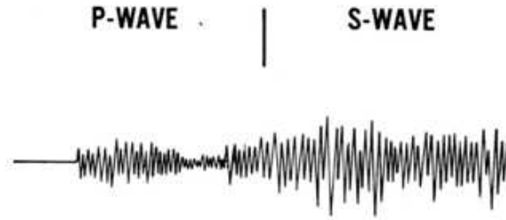
Figure 3.9: Graphical representation of the P- and S-wave arrival times.
