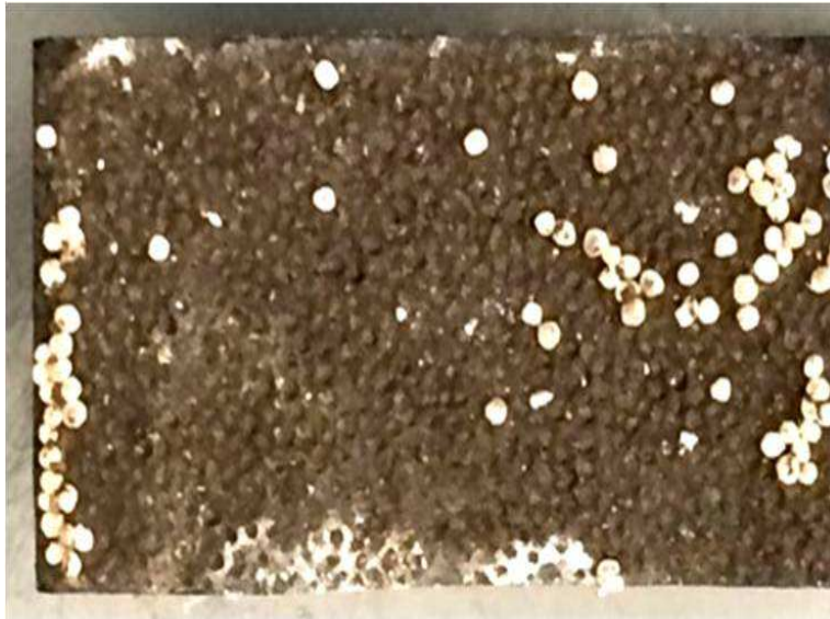
Figure 4.26: Vaca Muerta core sample showing the high level of indentation in the rock from proppant embedment after the triaxial stress conductivity experiment.
