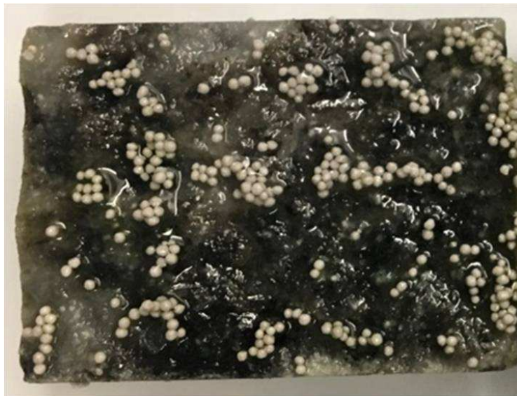
Figure 4.27: Niobrara core sample shown little to none proppant embedment after the triaxial stress conductivity experiment.
