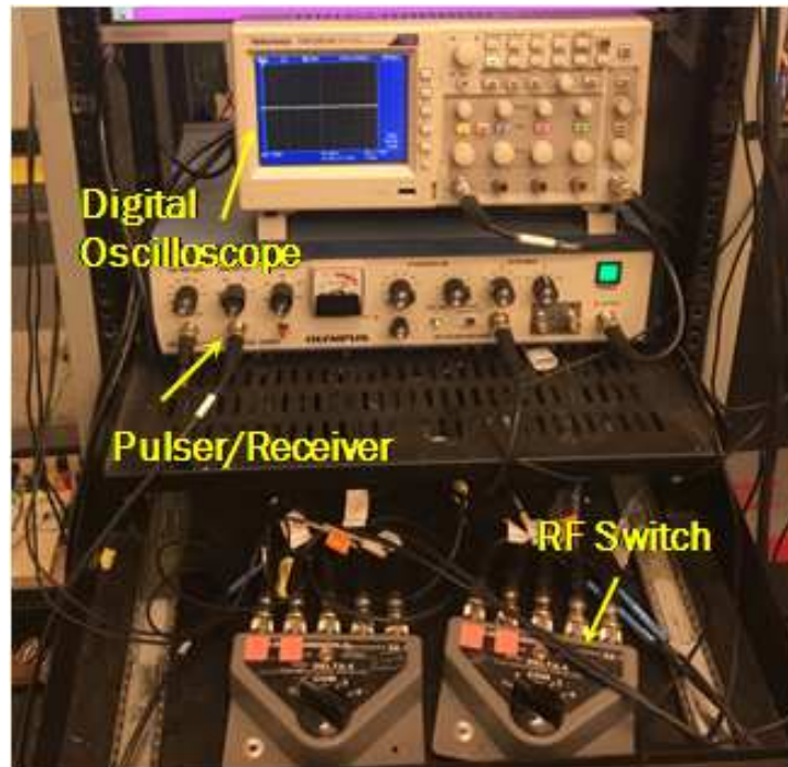
Figure 3.7: Digital oscilloscope, pulser/receiver and RF switch for selecting the measurement of P- and S-wave velocity.
