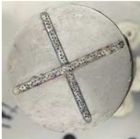
Figure 3.19: New porous filter to accommodate the low-pressure drop through the fractured core samples.
