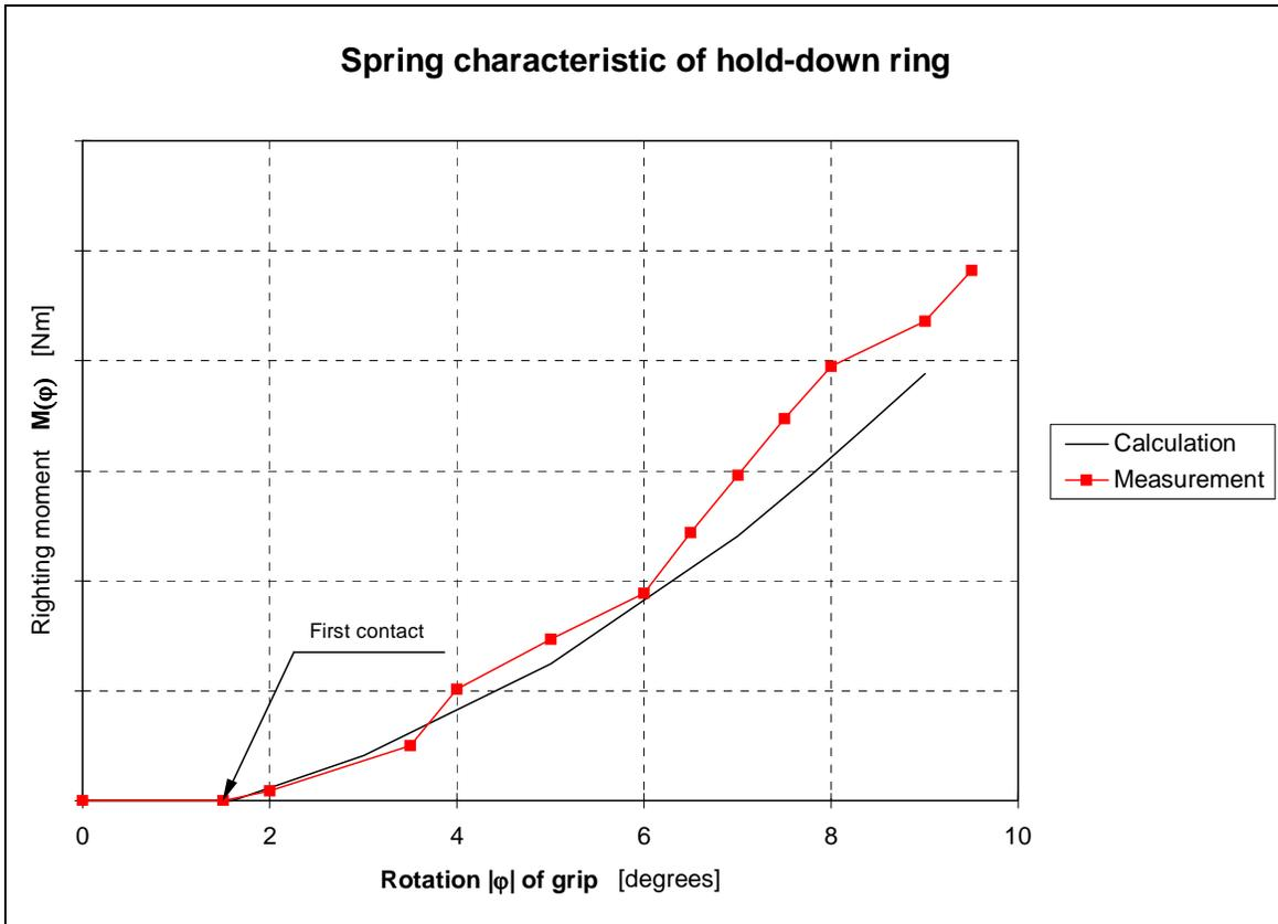
**Fig. 9:** Calculated hold-down ring characteristic
