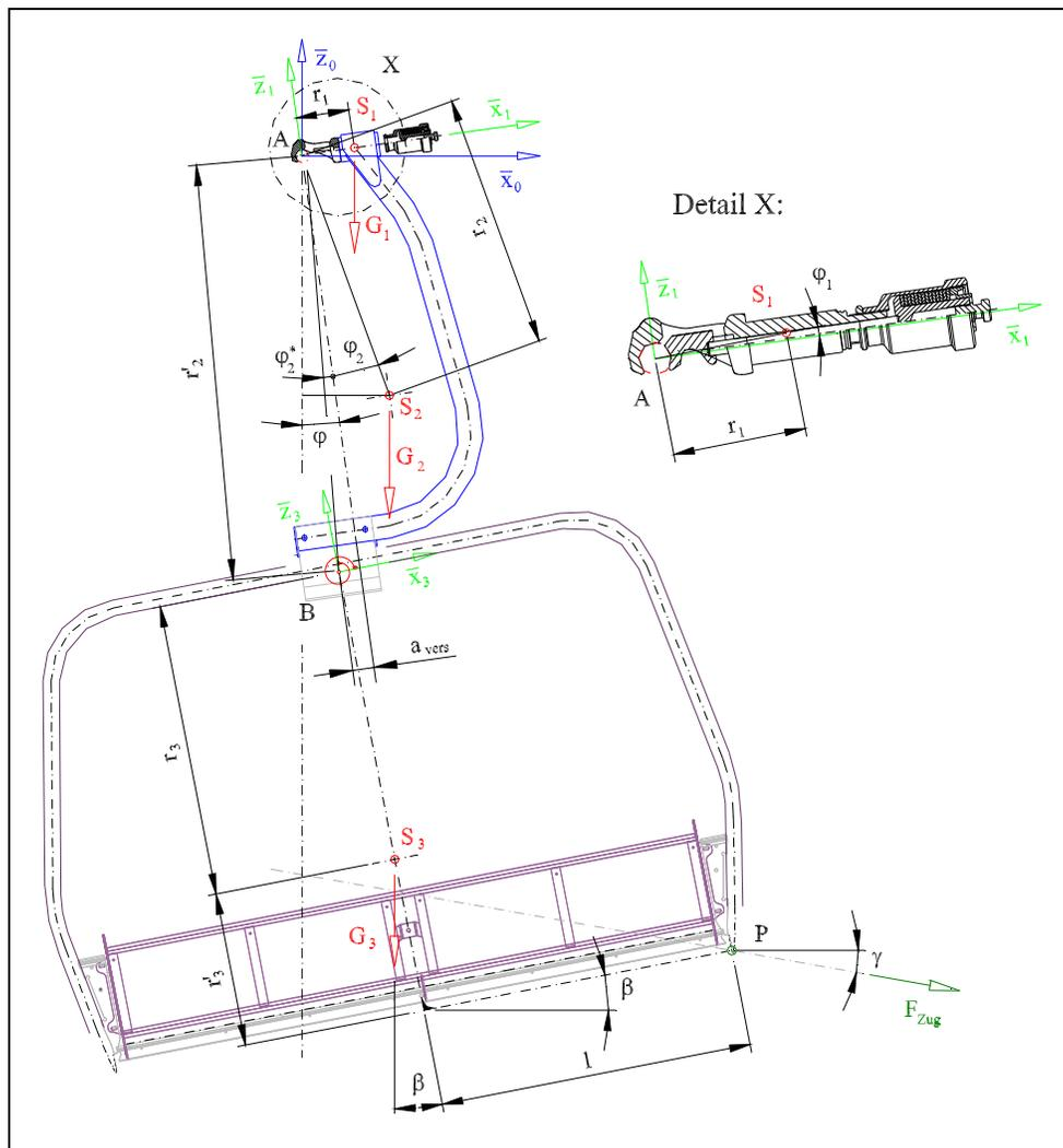
**Fig. 5:** Sketch of carrier pull test
