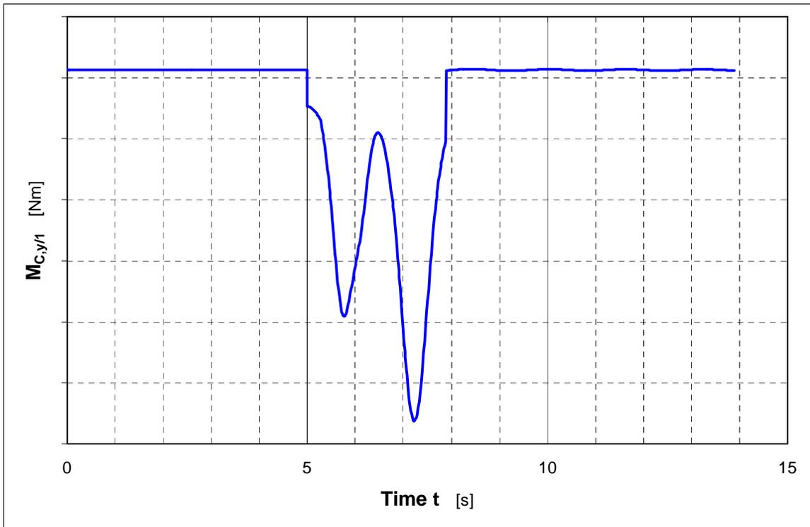
**Fig. 21:** Moment in joint C about the y axis, Load Case 6, rope speed  $v = 2.6$  m/s.
