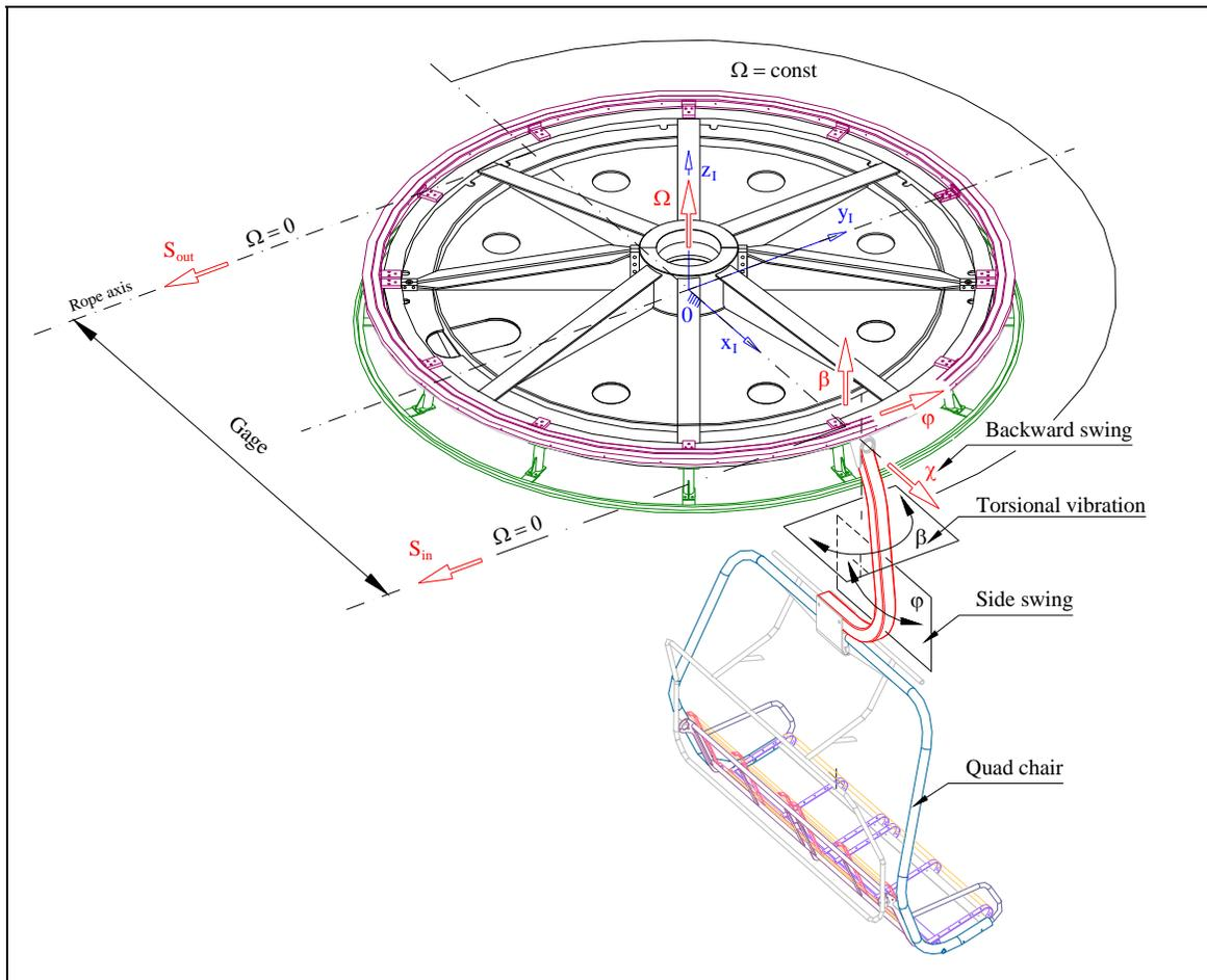
**Fig. 2:** What happens when a carrier passes around the bull wheel
