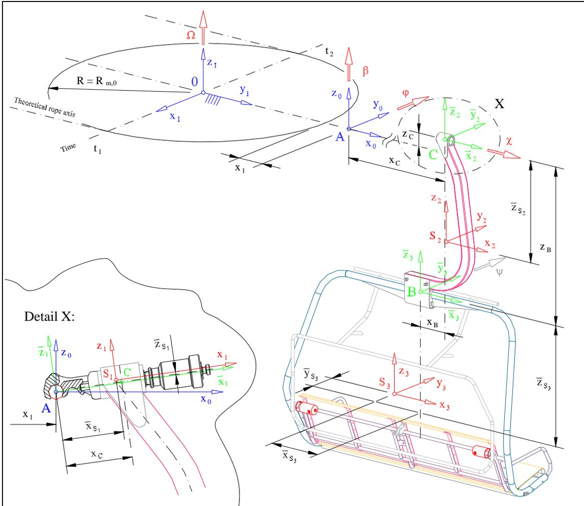
**Fig. 17:** Schematic of the geometrical configuration as the chair passes around the bull wheel
