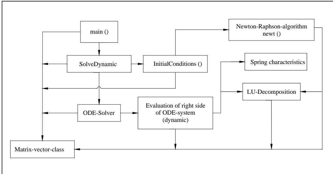
**Fig. 19:** Module hierarchy of the simulation program SIMCHAIR
