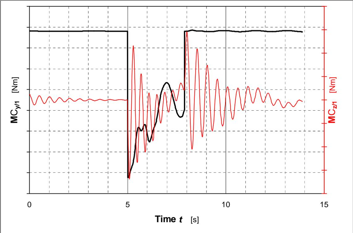
**Fig. 22:** Progression of moments in joint C for Load Case 5, rope speed of 2.6 m/s.
