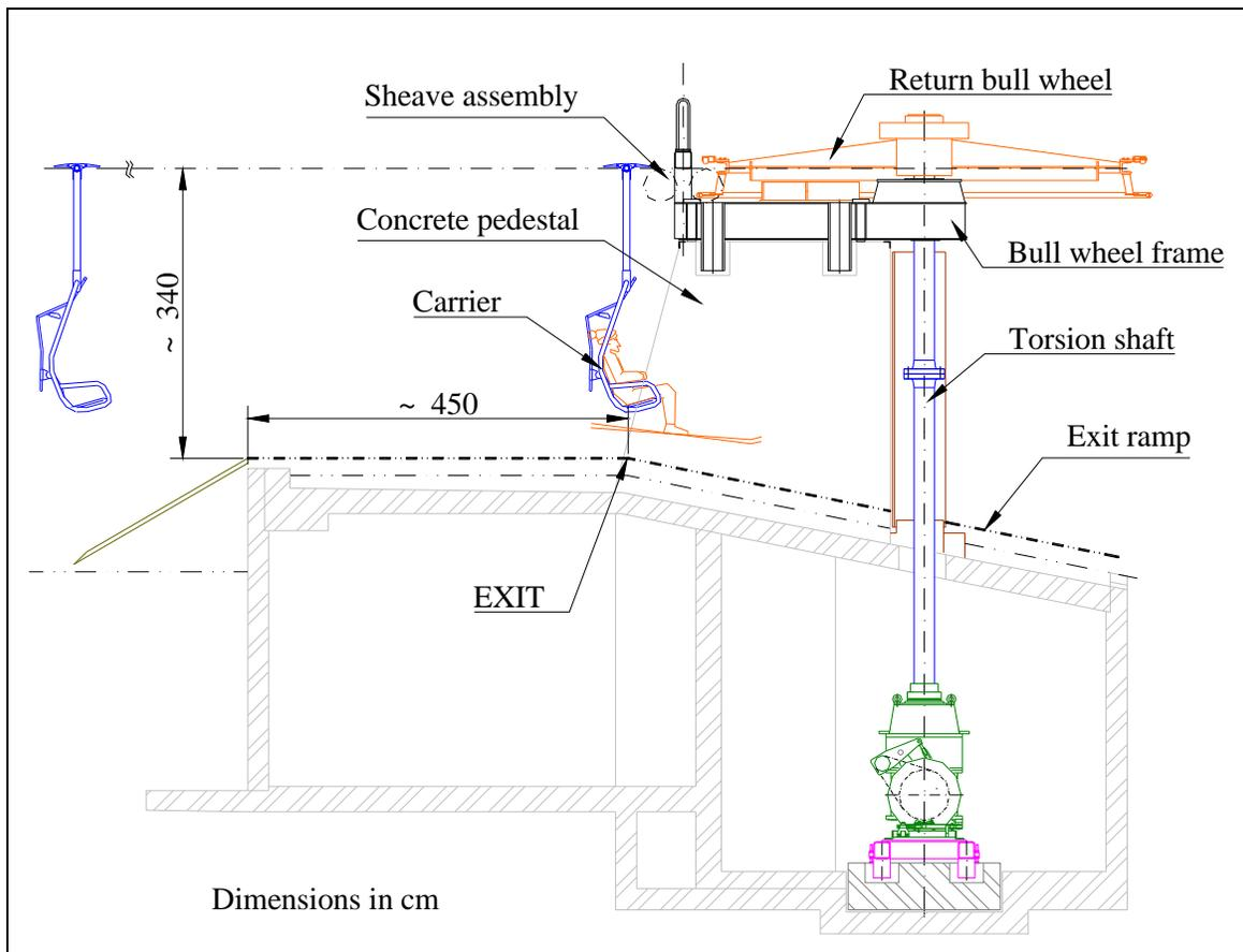
**Fig. 1:** Configuration of a bull wheel exit
