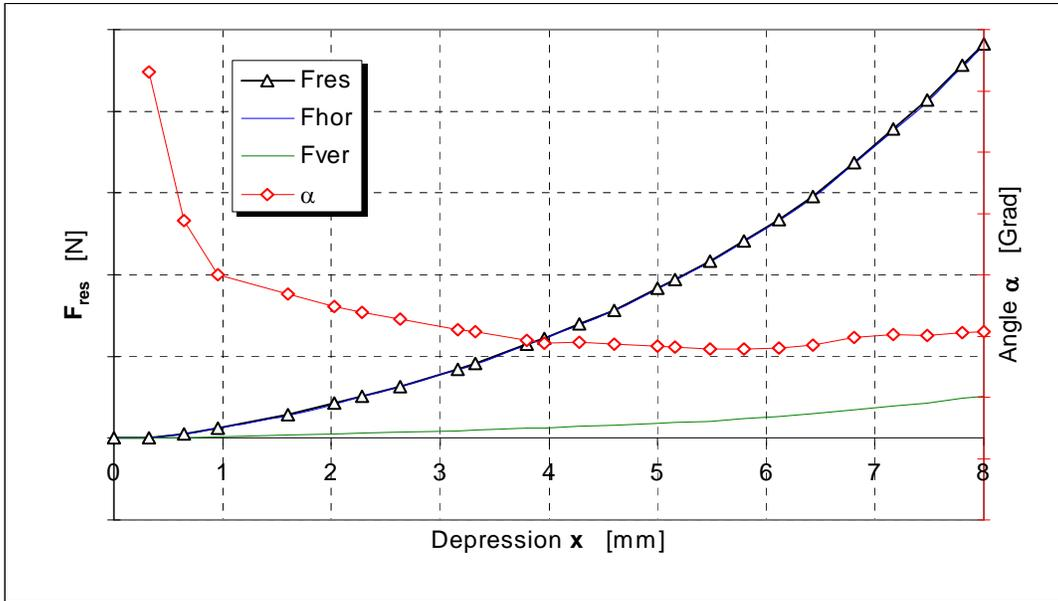
**Fig. 13:** Spring force  $F_{res}$  and angle in relation to depression of rubber by hanger arm
