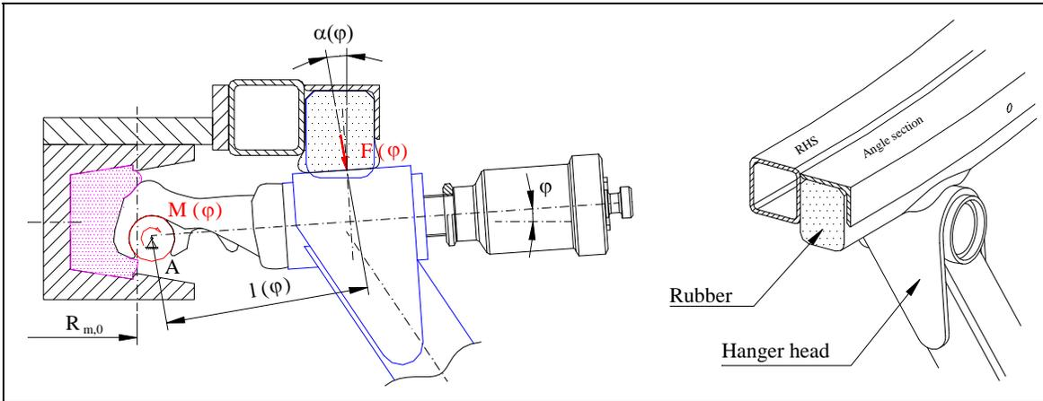
**Fig. 7:** Function schematic of the hold-down ring
