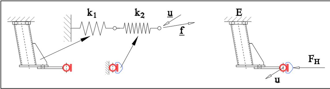
**Fig. 10:** Mechanical system for the guide ring
