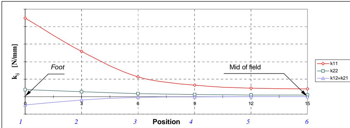
**Fig. 12:** Graphic representation of the individual matrix elements  $k_{ij}$ .
