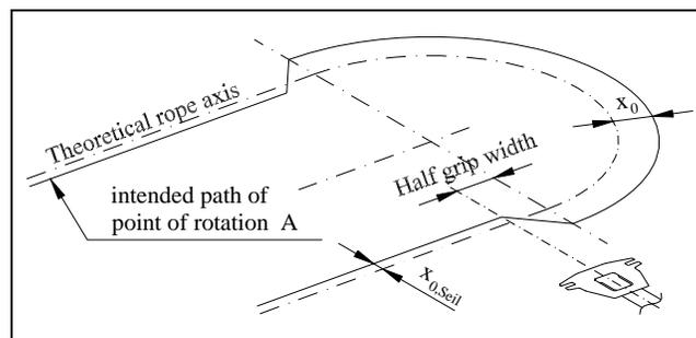
**Fig. 4:** Sketch of intended movement of point of rotation A
