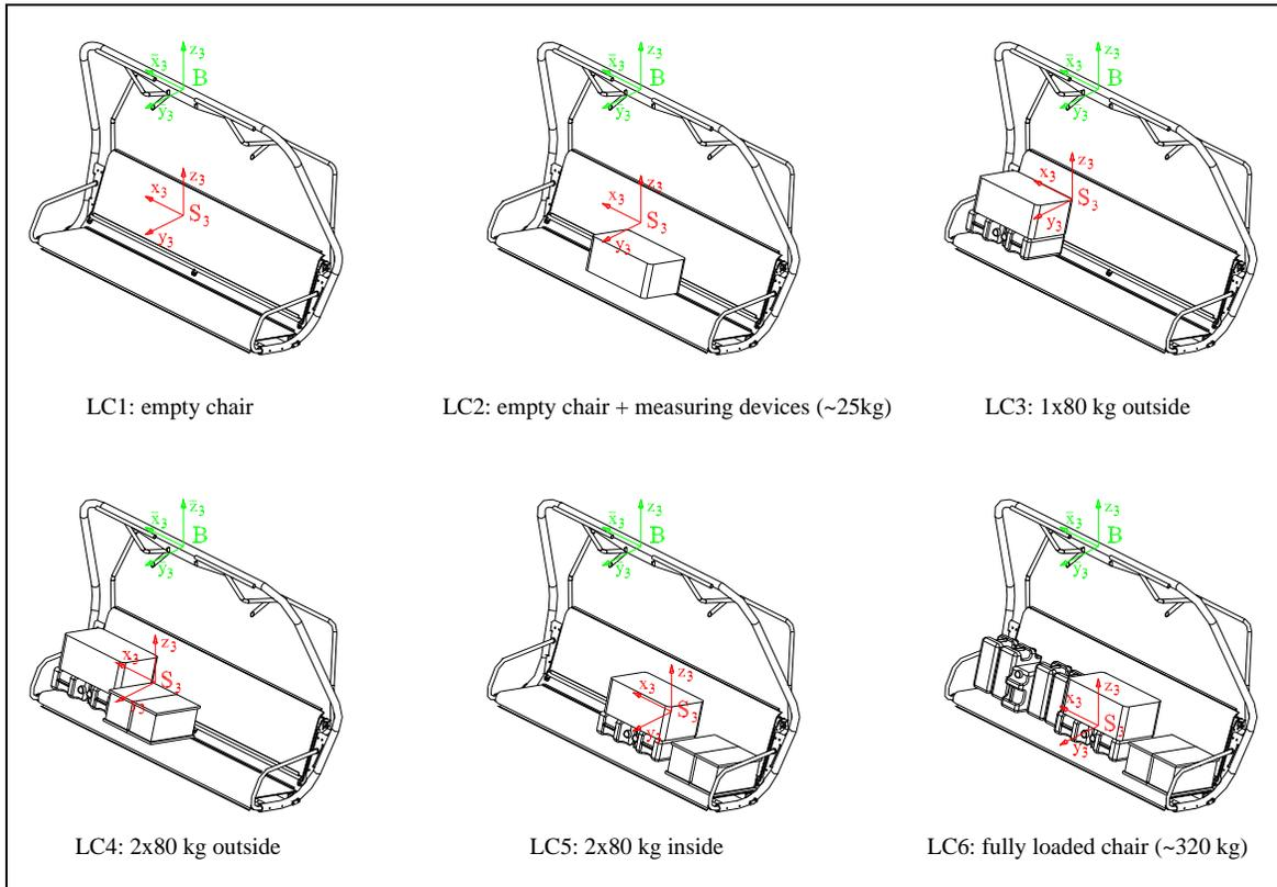
**Fig. 15:** Doppelmayr quad chair Model E / various load cases.
