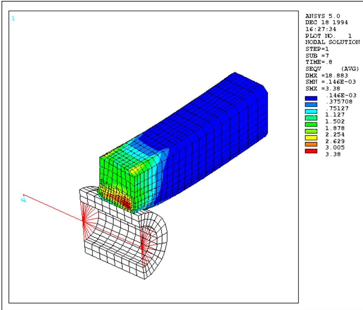
**Fig. 8:** Deformed FE model, von Mises stress in the rubber
