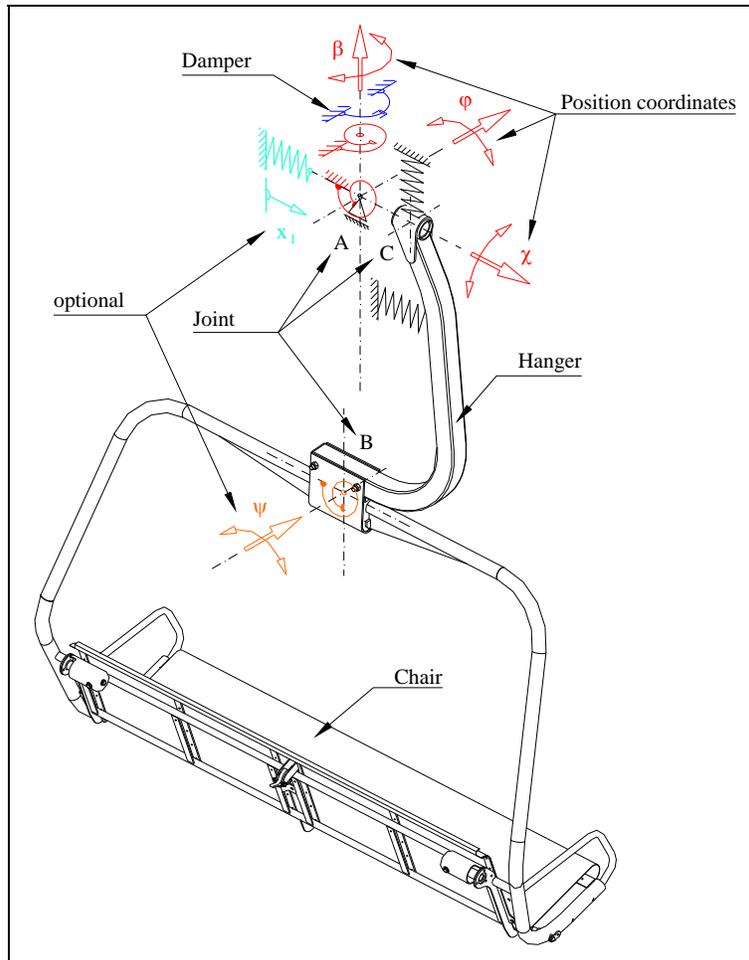
**Fig. 3:** Sketch of simulation model (rigid bodies, zero-mass springs)
