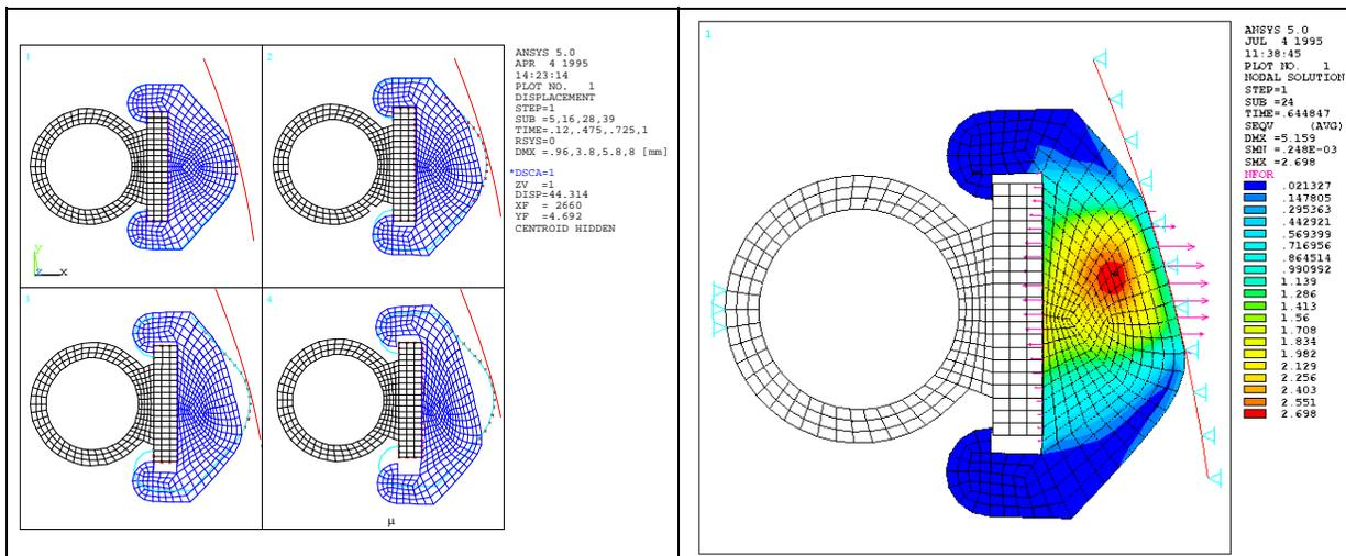
**Fig. 14:** Deformations of the FE model during various time increments of the calculation.
