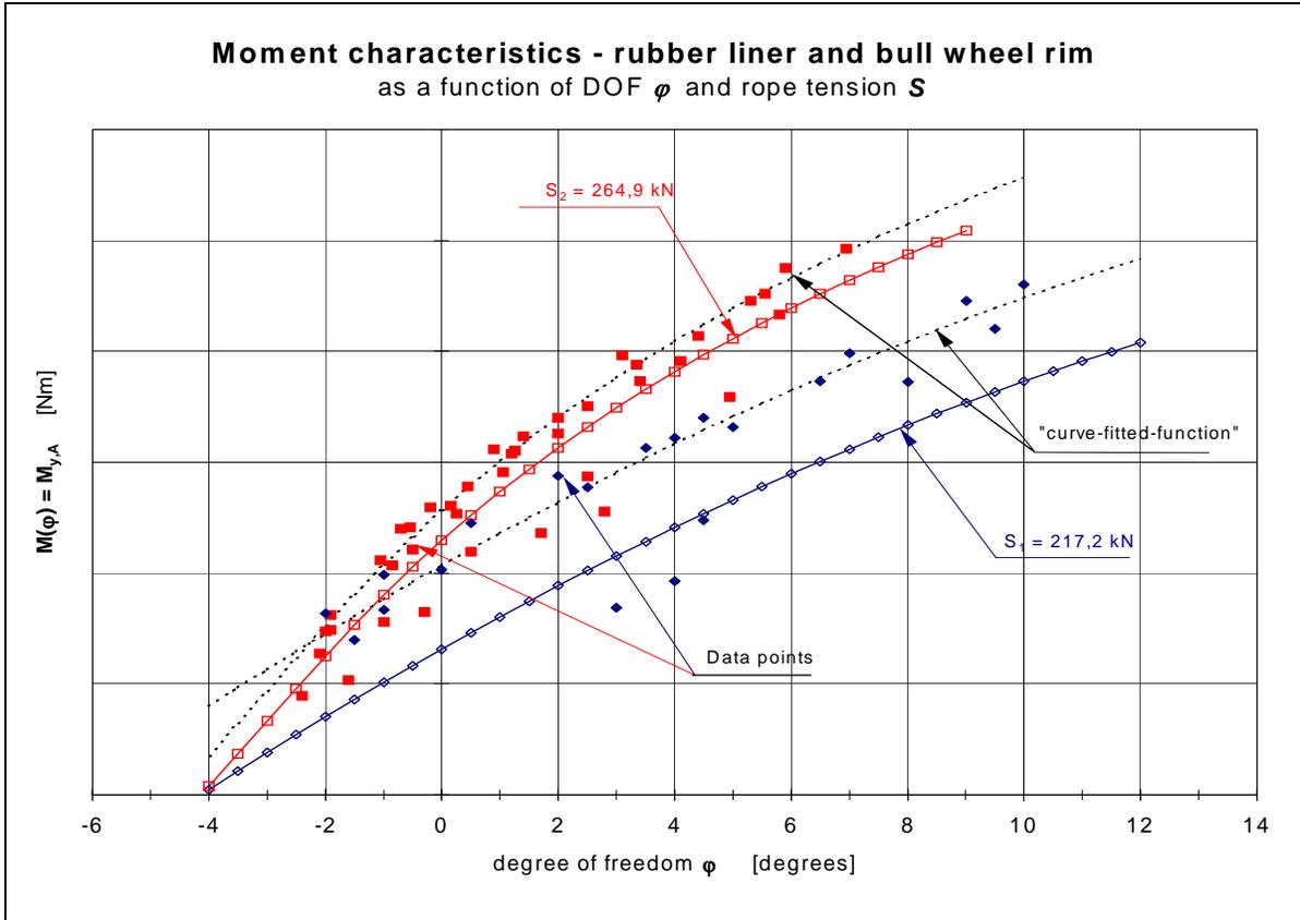
**Fig. 6:** Moment characteristics of the rubber liner
