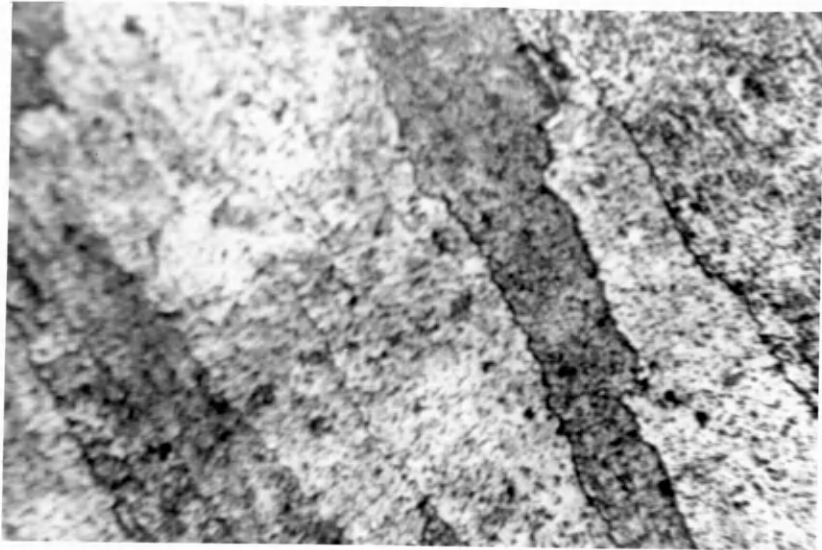
Figure 42. Ni/Al 2.3 + 20% Mo, B heat treatment. 700 x
