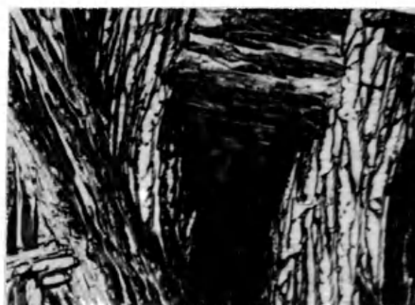
Figure 31. 5% iron 850x, 15 sec. etch.
