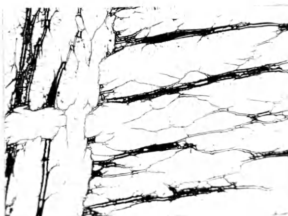
Figure 21. 1% iron 280x, 20 sec. etch.
