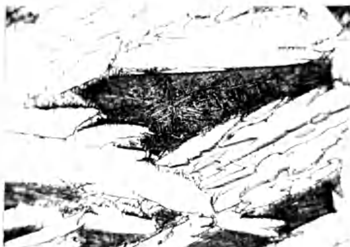
Figure 42. 1% iron 200x, 30 sec. etch.
