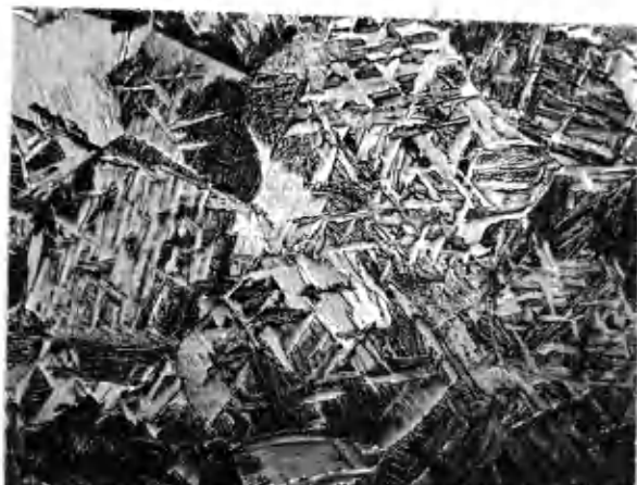
Figure 9. 1% iron 75x, 10 sec. etch. Annealed 1/2 hour at 1700 F.
