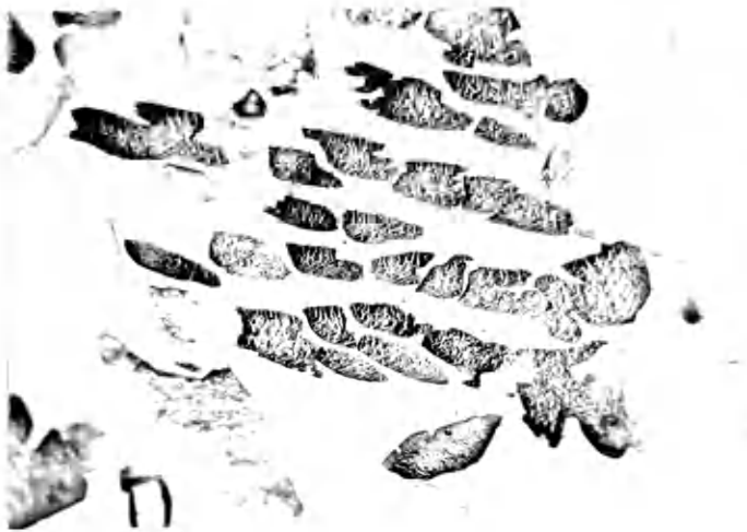
Figure 47. 5% iron 180x, 45 sec. etch.
