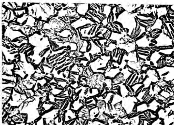
Figure 49. 10% iron 50x, 30 sec. etch. Quenched from 1700 F.
