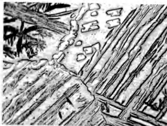
Figure 37. 10% iron 130x, 20 sec. etch.
