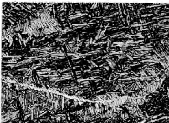
Figure 12. 2.5% iron 270x, 10 sec. etch.
