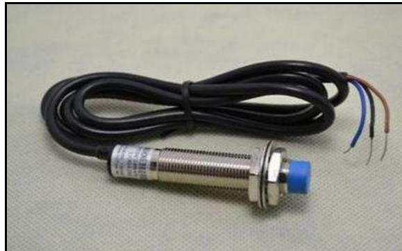
Figure A.14 Inductive proximity sensor PNP, 7 mm (0.27 in.) nominal sensing distance with a 0-10 V DC analog output.
