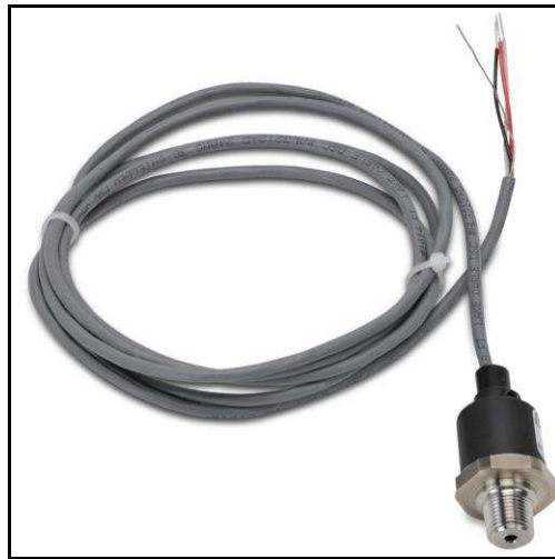
Figure A.12 ProSense waterproof pressure transmitter, 0 psig to 30 psig range with 0-10 V DC analog output, 14 V to 36 V DC operating voltage.
