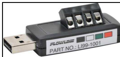
Figure A.8 Flowline Fob for USB interfaces with screw terminals.
