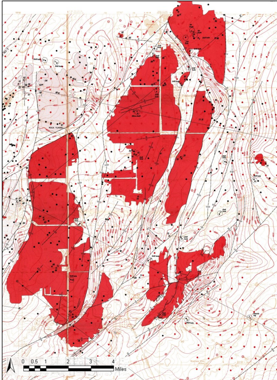
Figure 2.3: Regional faulting in the study area. Heavy NE trending faults (black lines) in the area influence known mine extents (red polygons) (Spencer, 1986).
