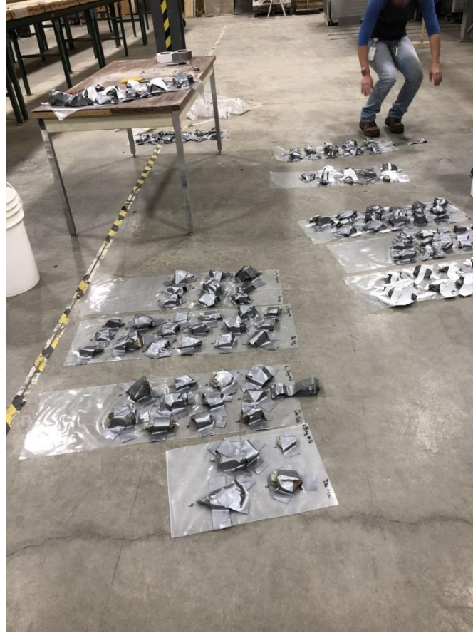
Figure 5.1: Sortation samples on tarps before XRT scanning.
