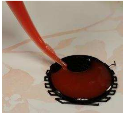
Figure 3.2: Manual Photopolymer Deposition Process
