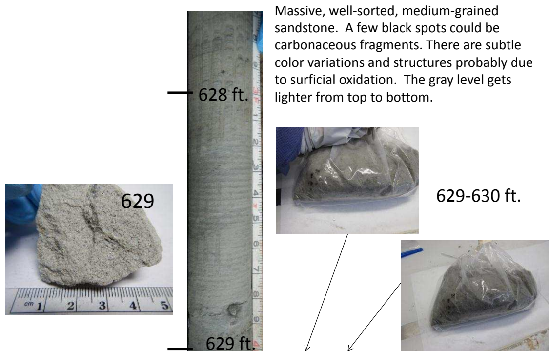
Figure 3.8: Photos of core material from 191.5 – 192.1 m below ground surface in borehole M3-2. Note that the interval used in column studies was 191.8 – 192.1 m, shown in the two plastic bags.
