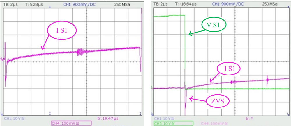
Fig. 5.11 a) Current waveform of switch 1. b) Current and voltage waveforms of switch 1 [33].
