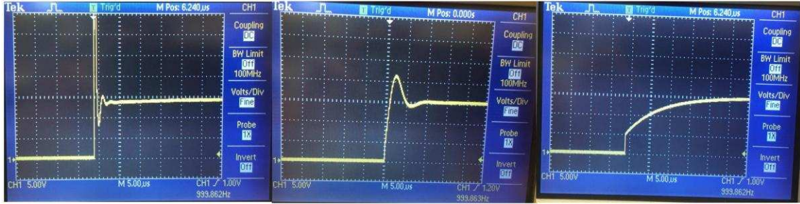
Figure 3. 15 Test result with capacitor value of (a)330pF (b)10nF (c)1µF.
