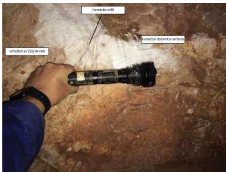
Figure 1.35. The Au9 dolomite lode vein. Euhedral dolomite faces are observed, and hematite fills in fractures.
