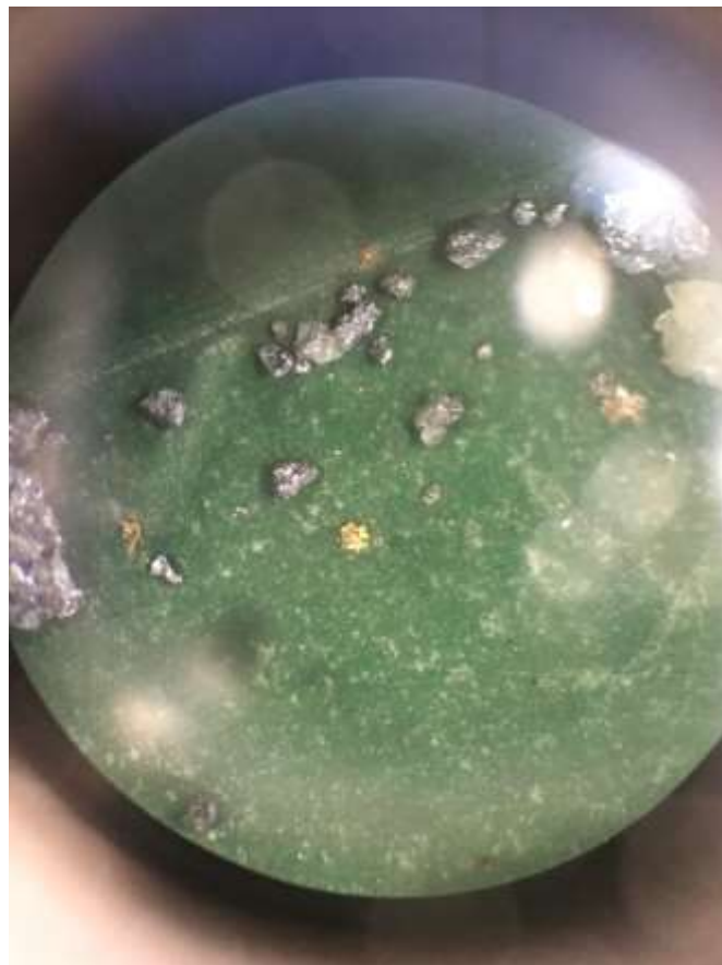
Figure E.1. Observable gold grains in hand-panned high-grade Au-Sb ore. Pictured is sample ZZG18-057 as viewed through binocular microscope. Approx. 40x magnification.
