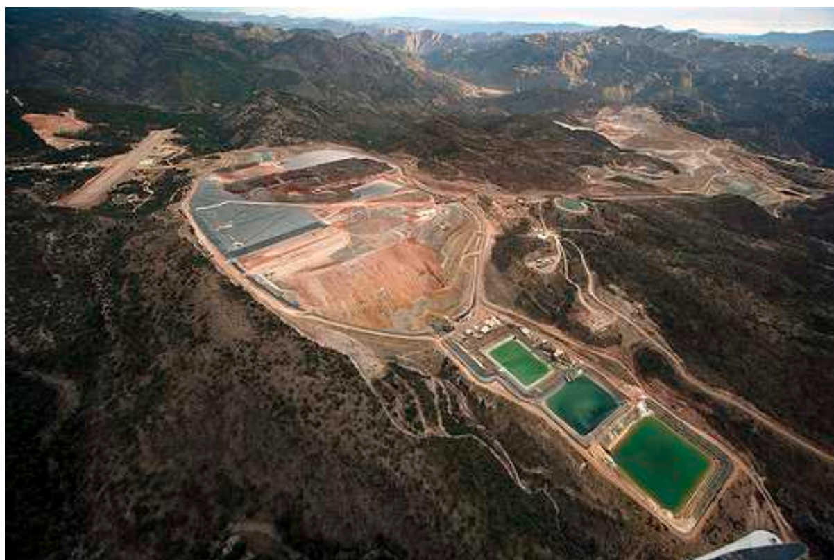
Figure 1.1: An aerial view of the Mulatos Gold Mine in Sonora Mexico. The hydrogen-cyanide pits are distinguishable by their characteristic green hue of resulting copper oxides [5]
