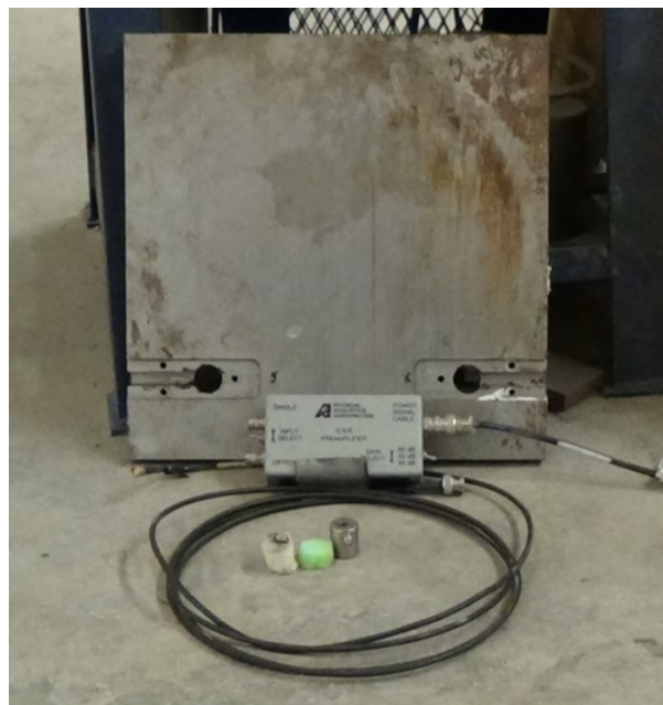
Figure 5: Platen, acoustic sensor with preamplifier, foam sleeve and backing
