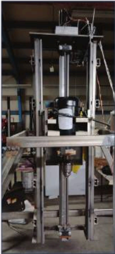
Drilling system fabricated by Deep Joshi and Dr. Bill Eustes to replicate drilling into analog and cryogenic lunar soil simulant. Images to left, above and below.
