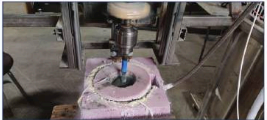
Drilling system fabricated by Deep Joshi and Dr. Bill Eustes to replicate drilling into analog and cryogenic lunar soil simulant. Images to left, above and below.
