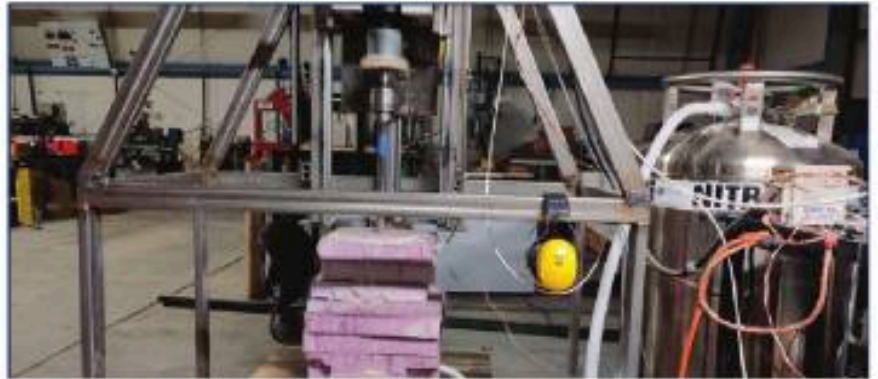
Drilling system fabricated by Deep Joshi and Dr. Bill Eustes to replicate drilling into analog and cryogenic lunar soil simulant. Images to left, above and below.
