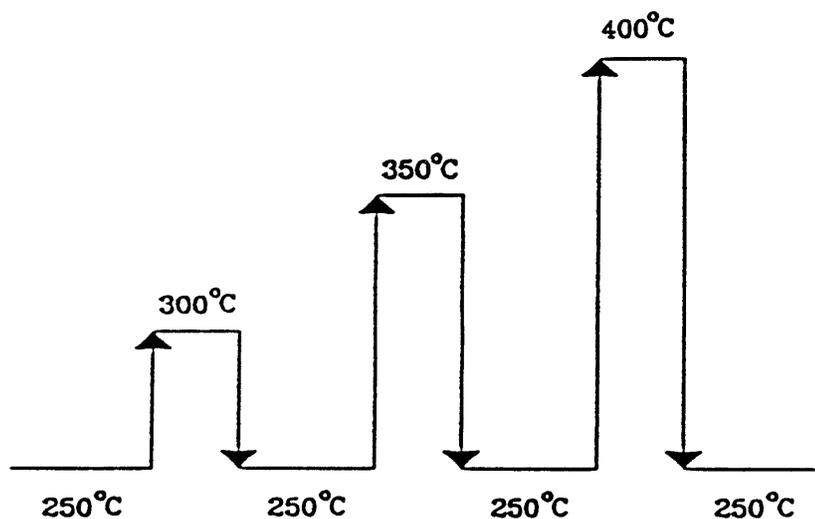
Figure 24. Temperature Pathway for the Stability Test
