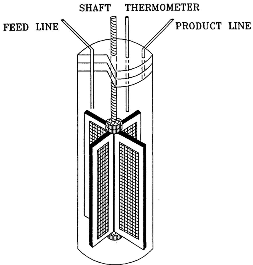
Figure 6. Cross-sectional View of the Reactor Internals.
