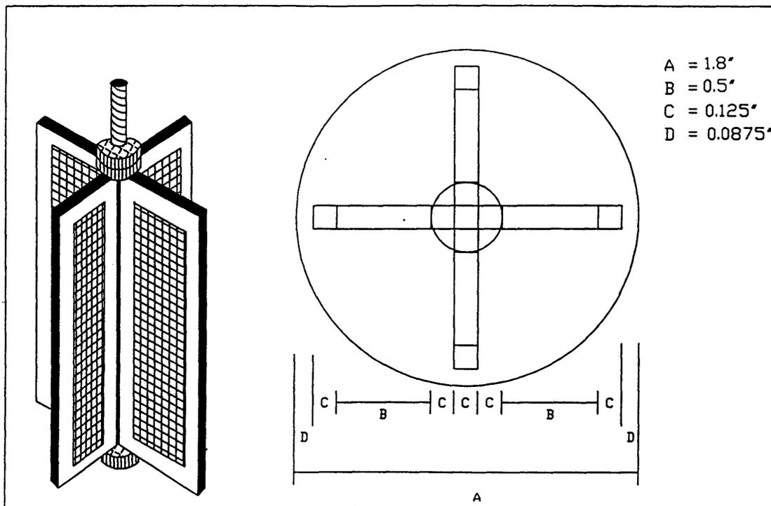
Figure 5. Detailed Dimensions of the Reactor Internals.
