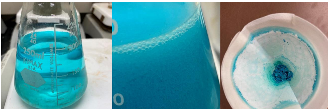
Figure 3.5: Copper Chloride wet chem method for determining sodium carbonate amount (left is the copper chloride solution, middle is the solid white precipitate formed by the reaction of sodium carbonate and copper chloride, and right is the filtered precipitate for analysis).
