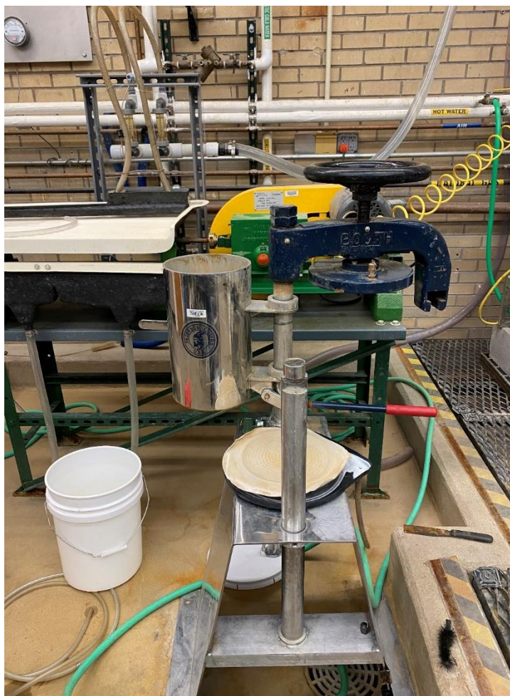
Figure 3.3: Laboratory pressure filter; the filter body and lid swing into place above the pad in the middle of the image
