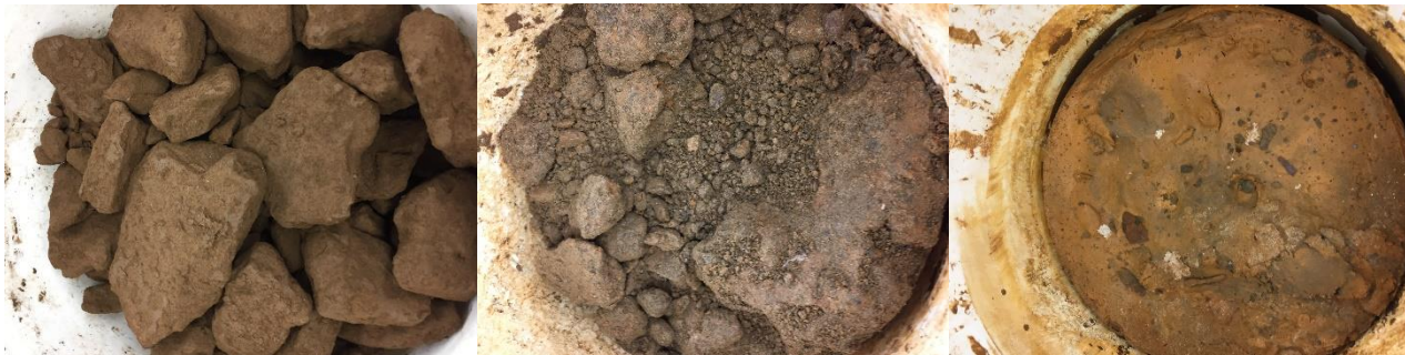
Figure 3.1: The CLP Sample used for this research was delivered in three pales, each having a different visual appearance, the first two containers had agglomerations covering a large cake like that seen in the third image.
