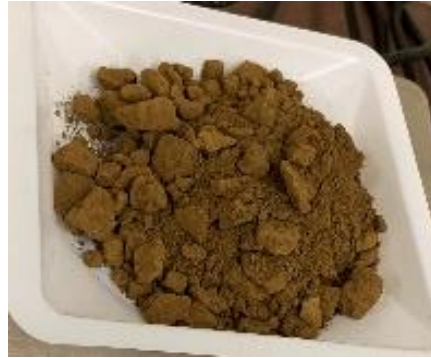
Figure 4.4: Picture of the CLP sample after crushing to break up large agglomerations
