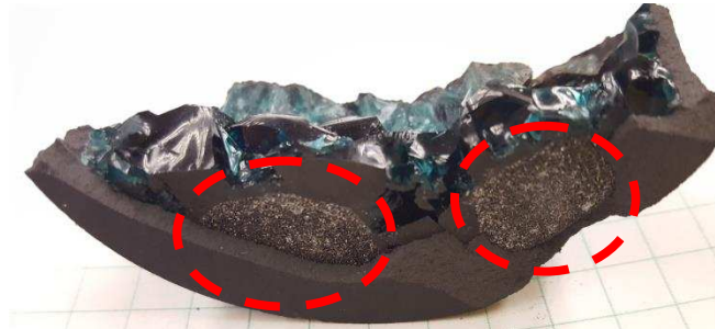
Figure 5.2 Bottom Face of Slag Contained in a Graphite Crucible. Regions of reduced iron are circled in red.
