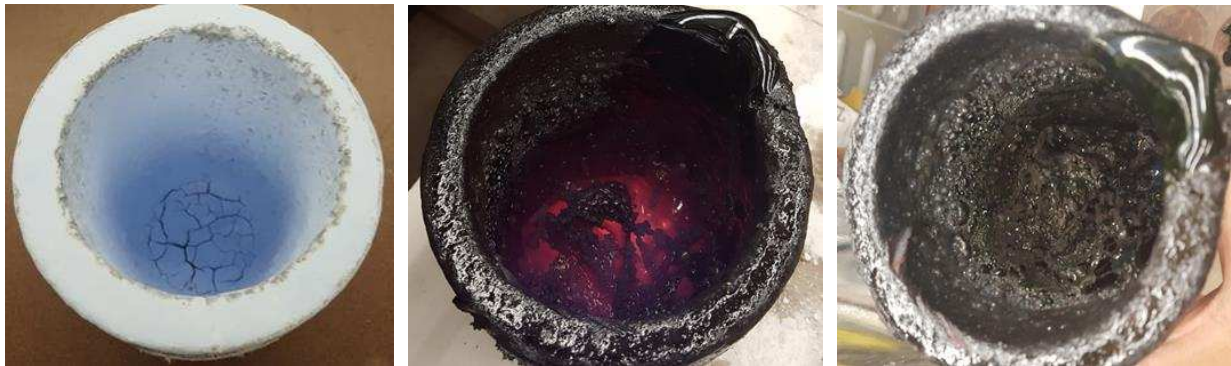
Figure 5.3 Silicon Carbide Crucible Coated with Boron Nitride. From left to right: before heating slag, immediately after heating slag to 1200 °C, and after cooling to room temperature.
