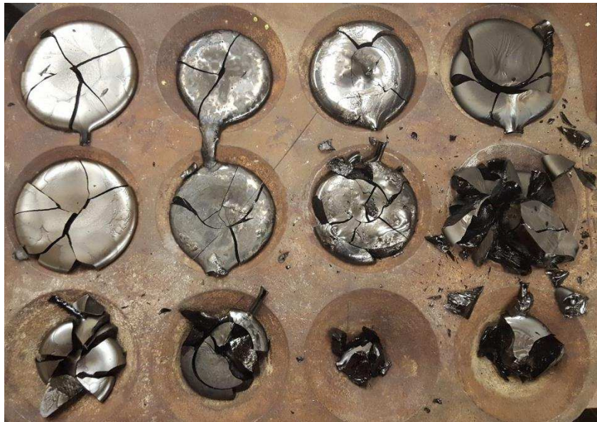
Figure 6.10 Poured Slags. From Left, Slags N, F, S, and M.
