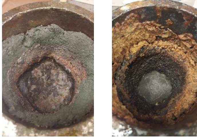
Figure 5.4 Two Crucibles Coated with Different Castable Refractory Compounds Containing a Slag, after heating.
