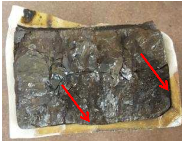
Figure 5.5 Alumina Crucible Containing a Slag After Heating. Discoloration due to slag wetting a crack is indicated with red arrows.
