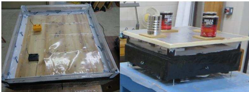
Figure 4.8: Impermeable Drying Experimental Setup
