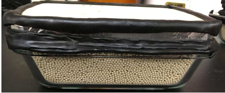
Figure 4.3: Water Vapor Permeance Experimental Assembly with Desiccant
